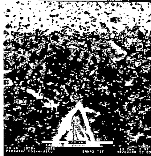
(b) The notch tip is located in an \text{Al}_2\text{O}_3 layer and there is no crack before a load is applied.
