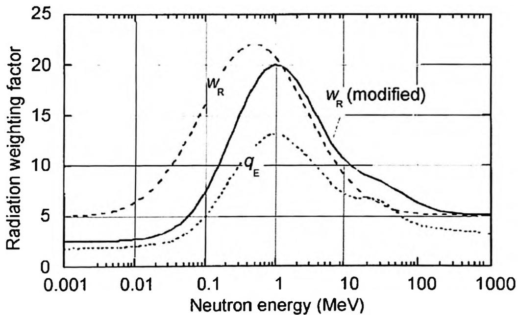
Figure 2.1: The current radiation weighting factor  $w_R$  (ICRP 60), the proposed modification  $w_R$  (modified) (ICRP 92), and the effective quality factor  $q_E$  for neutron radiation (ICRP, 2003).
