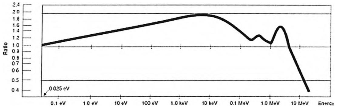
Figure 4.2: The energy dependent response of the SNOOPY (Canberra Instruments Inc., 2003).
