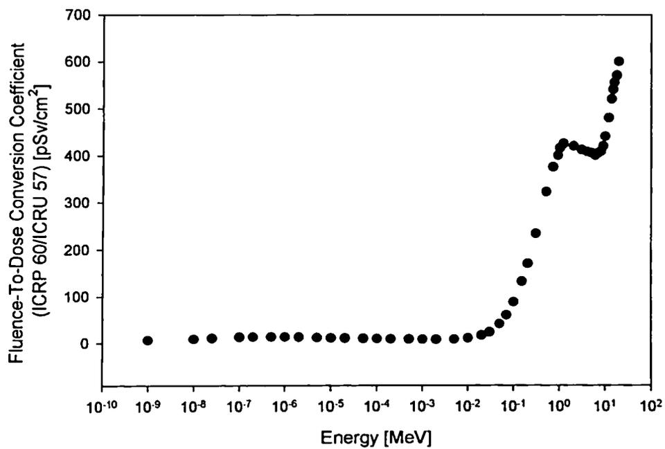
Figure 4.1: The Fluence-To-Dose Conversion Coefficients (ICPR 60/ICRU 57) (ICRP, 1991).
