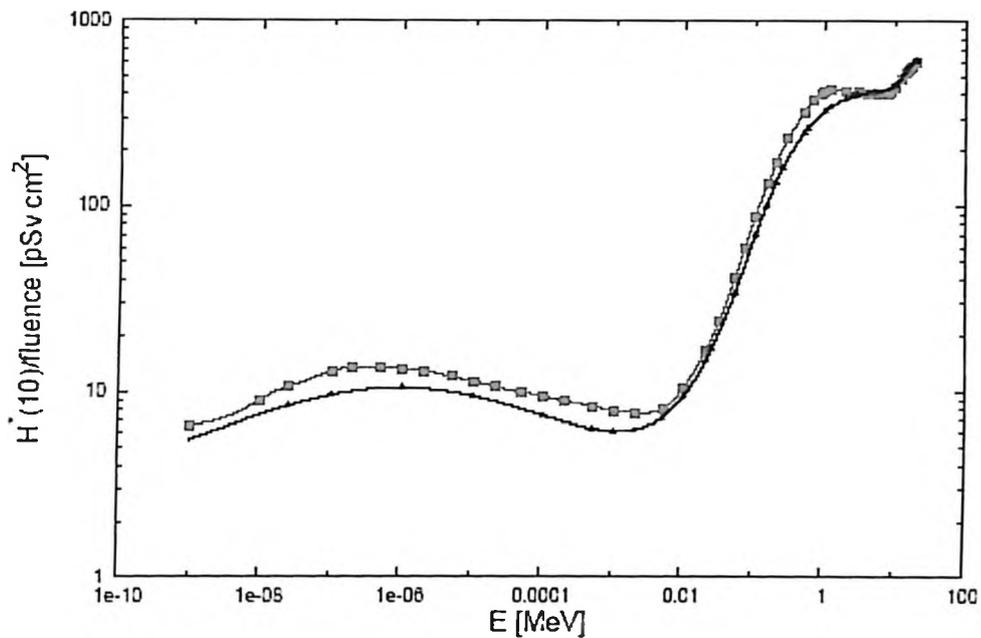
Figure 6.1: The neutron fluence to ambient dose conversion coefficients as a function of energy using values of quality factor (ICRP 26) as indicated by the triangle markings, and values of radiation weighting factor (ICRP 60) as indicated by the square markings (Saul and Ross, 2004).
