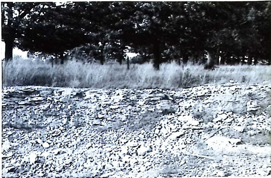
Illus. 18 The only quarry in the area of study. It is found in the Portie-Akron formation just north-west of Strouess. Note thin platy structure of strata. The material from this quarry was used in Port Maitland for road construction.
