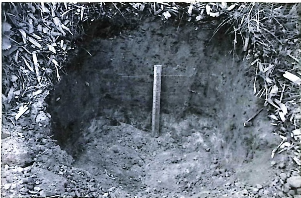
Illus. 14 Caister loam profile, showing a brown loam A horizon over a lighter brown sandy loam B horizon above a grey-brown gritty subsoil which starts about four inches from the bottom of the ruler.
