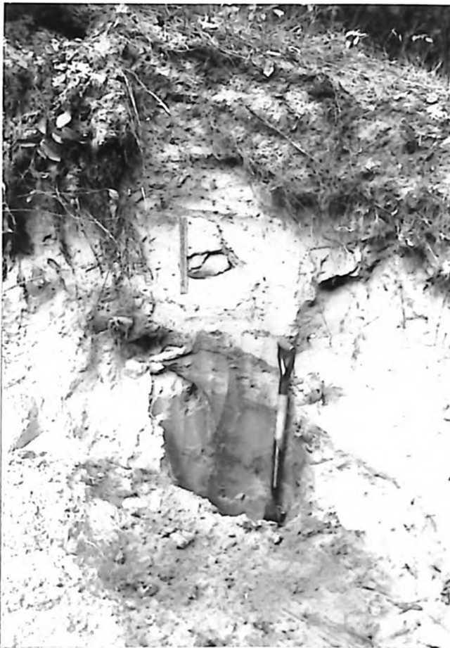
Illus. 10 Profile of Berrien sandy loam. Total depth is about seven feet. All material below the top of the ruler is pure sand and the dark zone near the spade is wet, showing the depth of the water table in the area. Profile was cut on the side of a sand dune.
