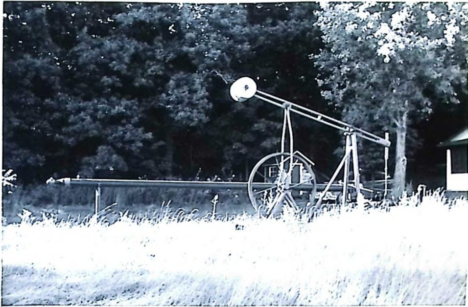
Illus. 20 A gas well on Mohawk Point. The machinery is used to pump water from the well. Behind is the cherry ridge (the top is just visible through the trees) of one of the moraine hills.
