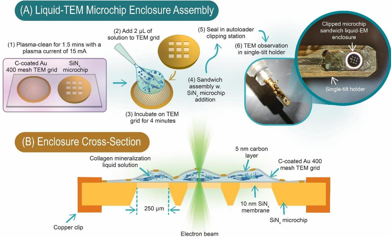
**Figure 1. Liquid-TEM microchip enclosure overview.** (A) Assembly process of the liquid-TEM microchip enclosure used for this research. (B) Enclosure cross-section with key dimensions.
