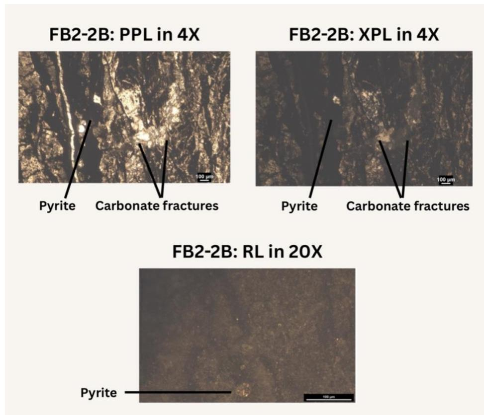
**Image 11.** Thin sections of fault rock 2 with slide 2B shown in plane-polarized light (PPL), cross-polarized light, and reflected light (RL).
