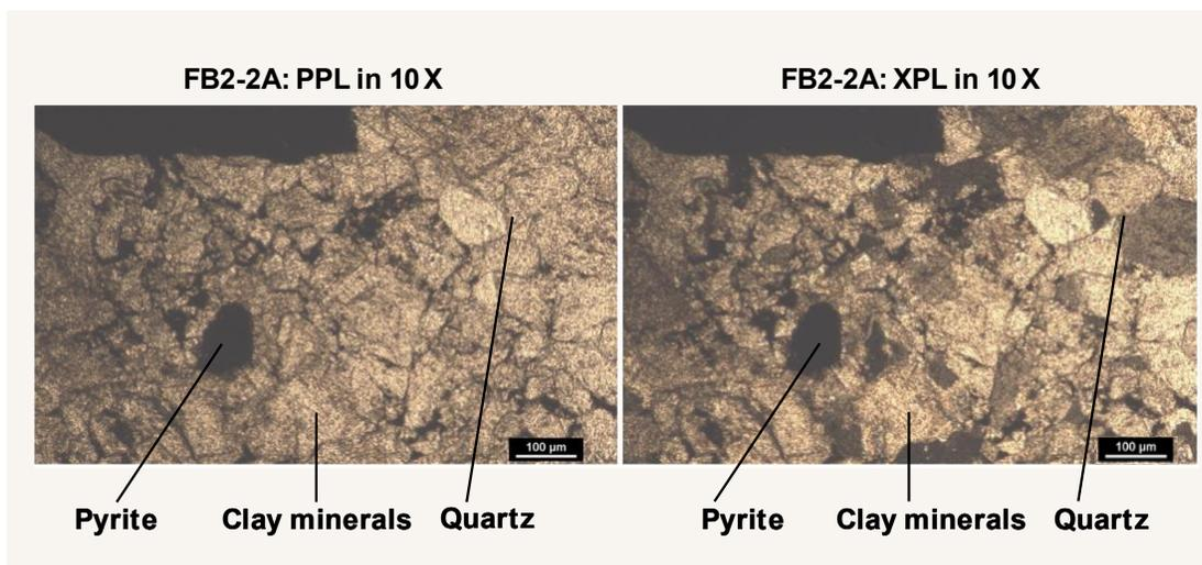
**Image 10.** Thin sections of fault rock 2 with slide 2A shown in plane-polarized light (PPL) and in cross-polarized light (XPL).
