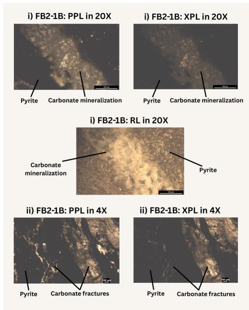
**Image 9.** Thin sections of fault rock 2 with slide 1B shown in plane-polarized light (PPL) (i, ii), cross-polarized light (XPL) (i, ii), and reflected light (RL) (i).
