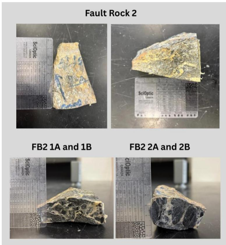
**Image 2.** Fault rock 2 (FB2) images showing rock thin section sides: FB2-1A and 1B, and FB2-2A and 2B.
