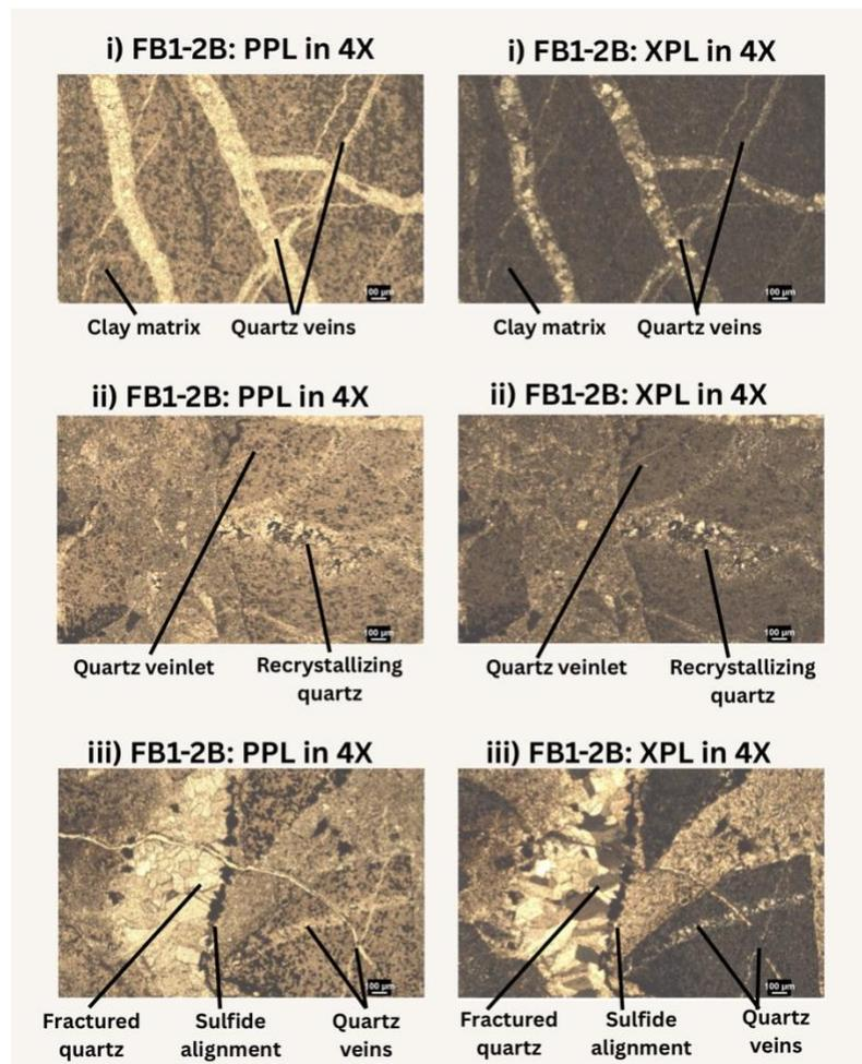
**Image 6.** Thin sections of fault rock 1 with slide 2B shown in plane-polarized light (PPL) (i, ii, iii), and cross-polarized light (XPL) (i, ii, iii).
