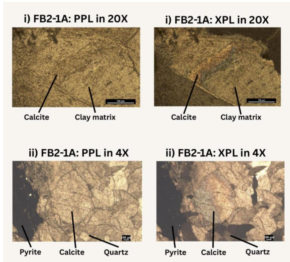
**Image 8.** Thin sections of fault rock 2 with slide 1A shown in plane-polarized light (PPL) (i, ii), and cross-polarized light (XPL) (i, ii).
