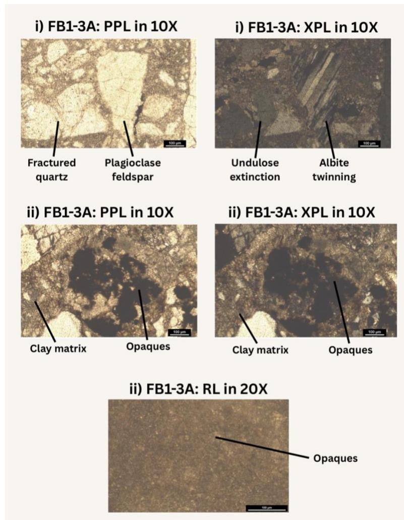
**Image 7.** Thin sections of fault rock 1 with slide 3A shown in plane-polarized light (PPL) (i, ii), cross-polarized light (XPL) (i, ii), and reflected light (RL) (ii).
