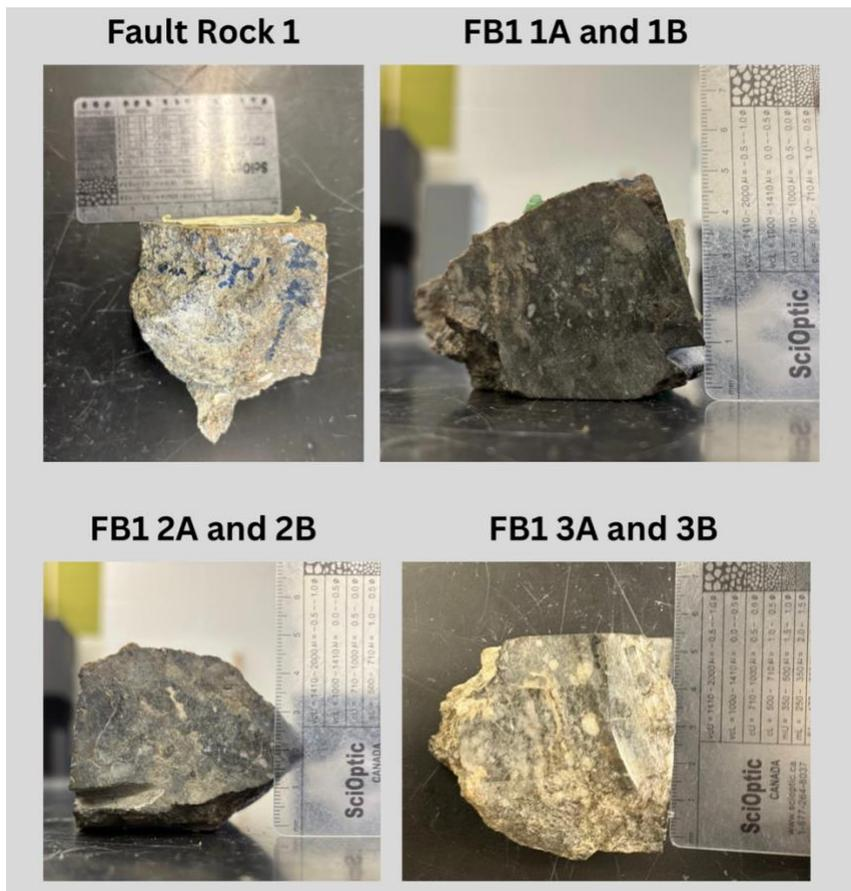
**Image 1.** Fault rock 1 (FB1) images showing rock thin section sides: FB1-1A and 1B, FB1-2A and 2B, and FB1-3A and 3B.
