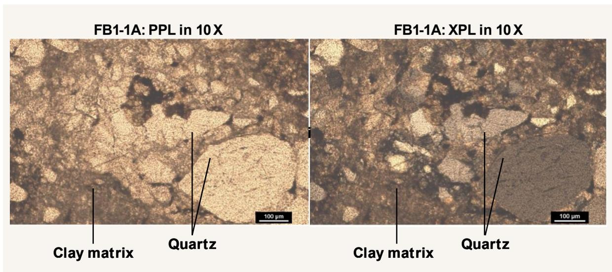
**Image 3.** Thin sections of fault rock 1 with slide 1A shown in plane-polarized light (PPL) and in cross-polarized light (XPL).
