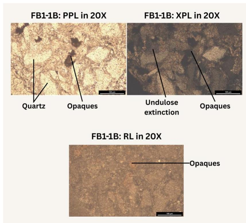
**Image 4.** Thin sections of fault rock 1 with slide 1B shown in plane-polarized light (PPL), cross-polarized light (XPL), and reflected light (RL).
