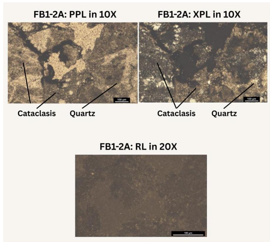
**Image 5.** Thin sections of fault rock 1 with slide 2A shown in plane-polarized light (PPL), cross-polarized light (XPL), and reflected light (RL).
