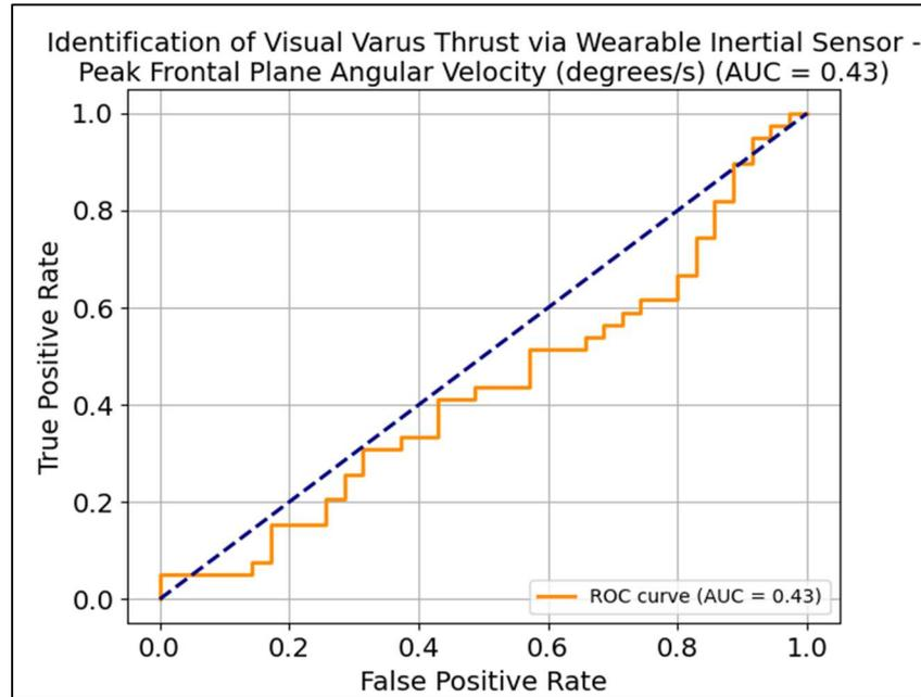
Figure 20: The ROC curve illustrates the diagnostic performance of the wearable inertial sensor (peak frontal plane tibial angular velocity in degrees/s) in detecting varus thrust. The area under the curve (AUC) is 0.43, indicating failure in discriminatory ability. The dashed diagonal line represents the line of no discrimination (AUC = 0.5).
