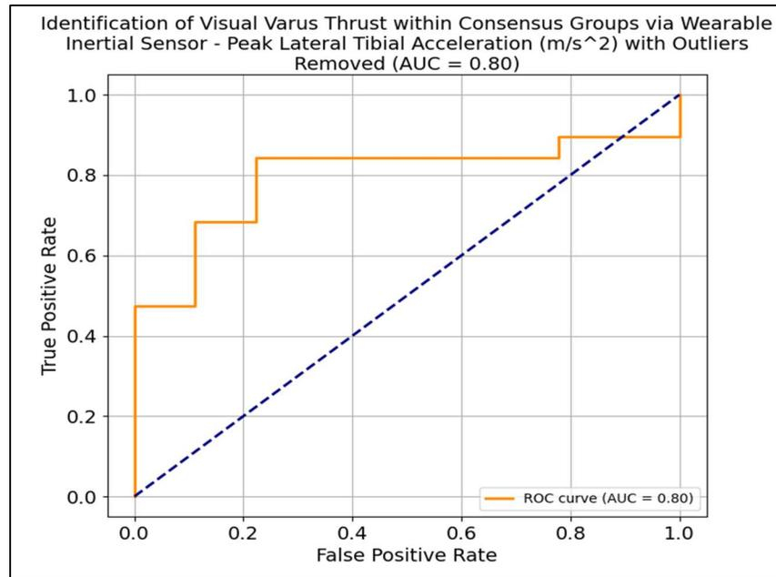
Figure 18: The ROC curve illustrates the diagnostic performance of the wearable sensor (peak lateral tibial acceleration in  $m/s^2$ ) in detecting varus thrust, for the consensus group with outliers removed. The area under the curve (AUC) is 0.80 indicating good discriminatory ability. The dashed diagonal line represents the line of no discrimination (AUC = 0.5).
