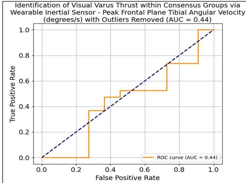
Figure A4: The ROC curve illustrates the diagnostic performance of the wearable sensor system (gyroscope) in detecting varus thrust, for the consensus group with outliers removed. The area under the curve (AUC) is 0.44, indicating failure in discriminatory ability. The dashed diagonal line represents the line of no discrimination (AUC = 0.5)
