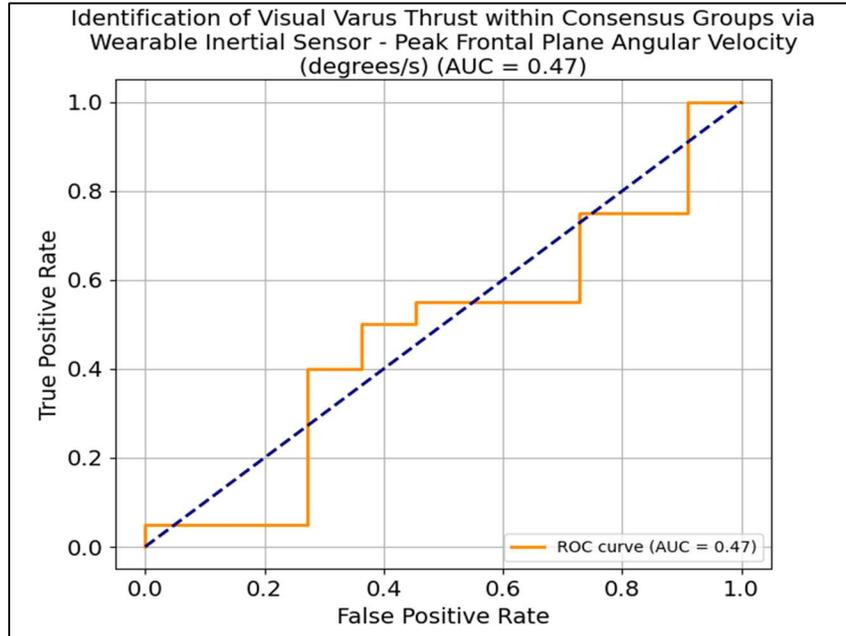
Figure 22: The ROC curve illustrates the diagnostic performance of the wearable sensor system (peak frontal plane tibial angular velocity in degrees/s) in detecting varus thrust, for the consensus group. The area under the curve (AUC) is 0.47, indicating a discriminatory ability worse than random chance. The dashed diagonal line represents the line of no discrimination (AUC = 0.5).
