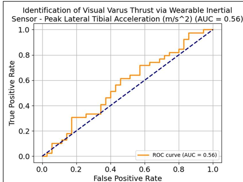
Figure 15: The ROC curve illustrates the diagnostic performance of the tibial inertial sensor (peak lateral tibial acceleration in  $m/s^2$ ) in detecting varus thrust. The area under the curve (AUC) is 0.56, indicating failure in discriminatory ability. The dashed diagonal line represents the line of no discrimination (AUC = 0.5).
