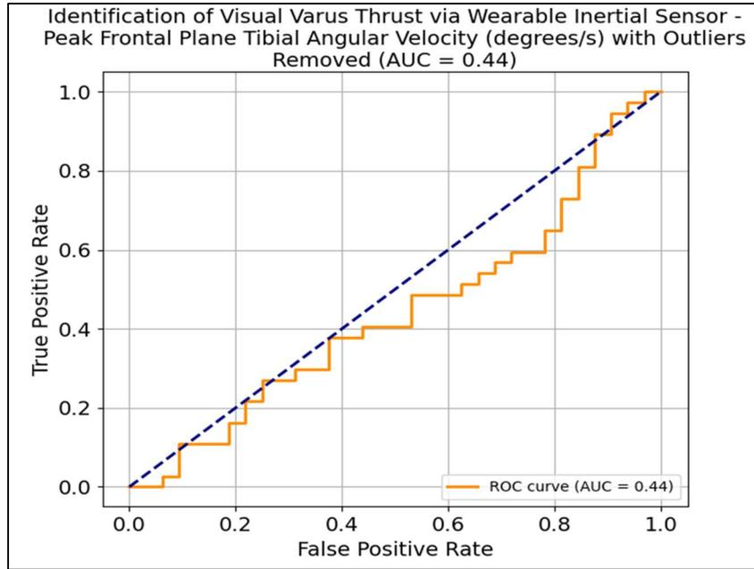
Figure A2: The ROC curve illustrates the diagnostic performance of the wearable inertial sensor system (gyroscope) in detecting varus thrust, for the full participant pool with outliers removed. The area under the curve (AUC) is 0.44, indicating a discriminatory ability worse than random chance. The dashed diagonal line represents the line of no discrimination (AUC = 0.5).
