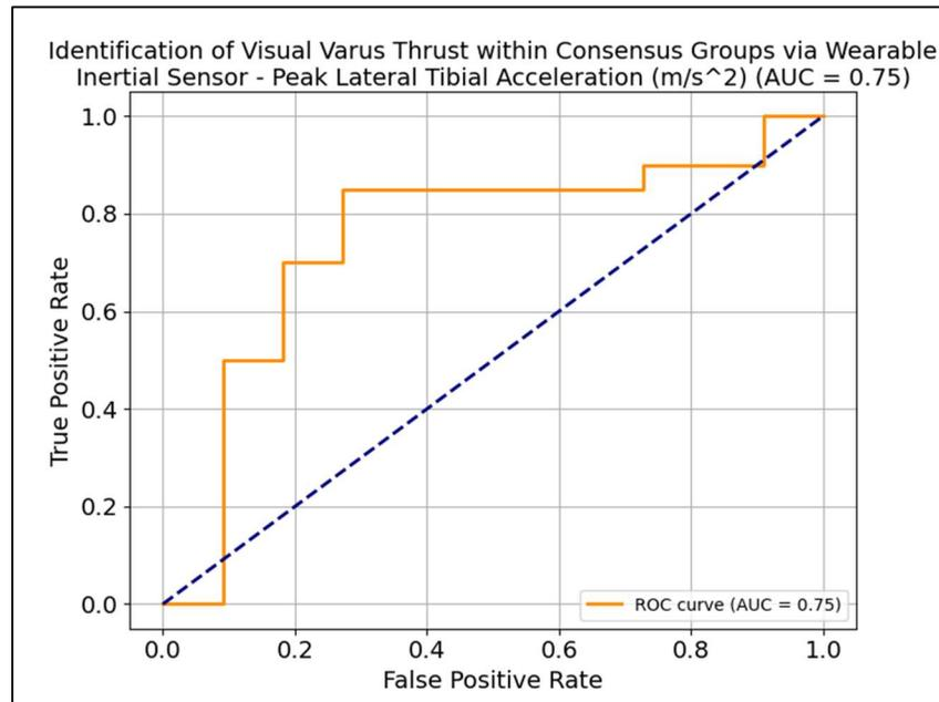
Figure 17: The ROC curve illustrates the diagnostic performance of the wearable sensor (peak lateral tibial acceleration in  $m/s^2$ ) in detecting varus thrust, for the consensus group. The area under the curve (AUC) is 0.75 indicating fair discriminatory ability. The dashed diagonal line represents the line of no discrimination (AUC = 0.5).
