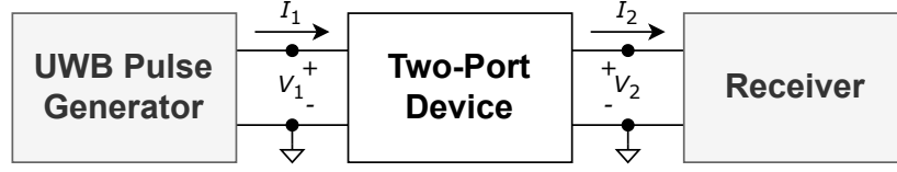
Figure 3.15: The two-port device representing a directional coupler in the measurements with the time-sampling receivers.
