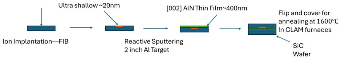
Figure 3.2. Schematic diagram of Ga implantation and activation process
