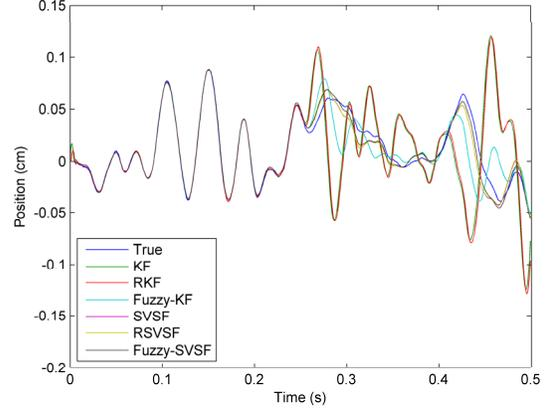
**Fig. 3.** EHA estimation results for all six filtering strategies, for the fault case. The modeling uncertainty is injected half-way through the simulation. The SVSF-based methods yield the most accurate results in this case.
