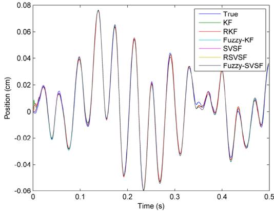
**Fig. 2.** EHA estimation results for all six filtering strategies, for the normal case. All filters are able to follow the trajectory well.
