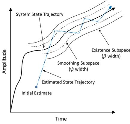
**Fig. 2b.** Chattering is present during the SVSF estimation process when the smoothing subspace is defined too small [10]. In this case, not all of the uncertainties have been considered.
