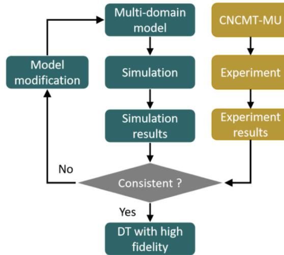
Figure 1. Consistency retention / model validation process<sup>20</sup>
