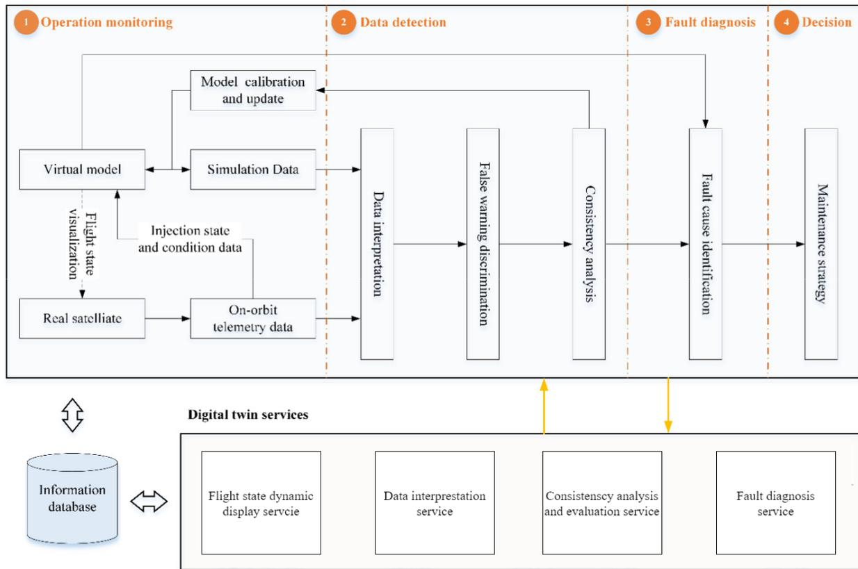
Figure 3. Example of a DT for satellites for fault detection from<sup>24</sup>
