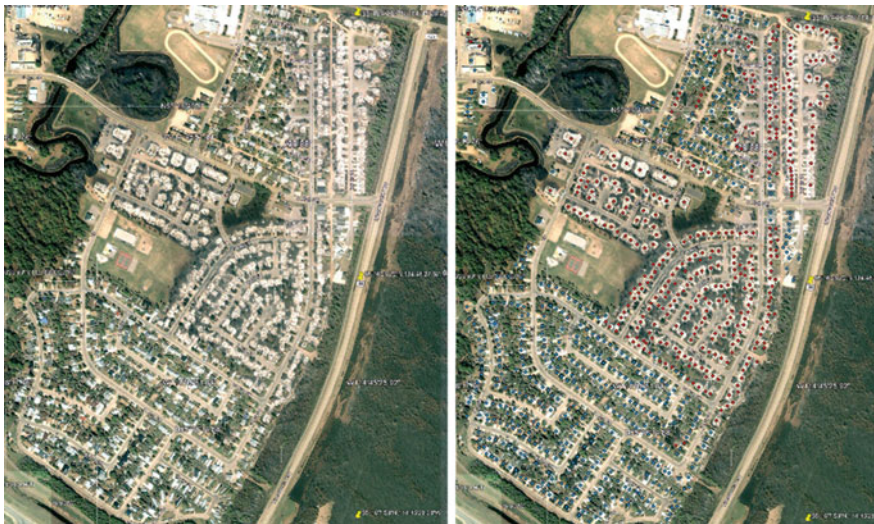
Fig. 3 Satellite image (Google earth pro©.) of part of the community of Slave Lake taken after the fire shown on the left image and the georeferenced destroyed (in red) and survived (in blue) buildings shown on the right image in ArcGIS © software
