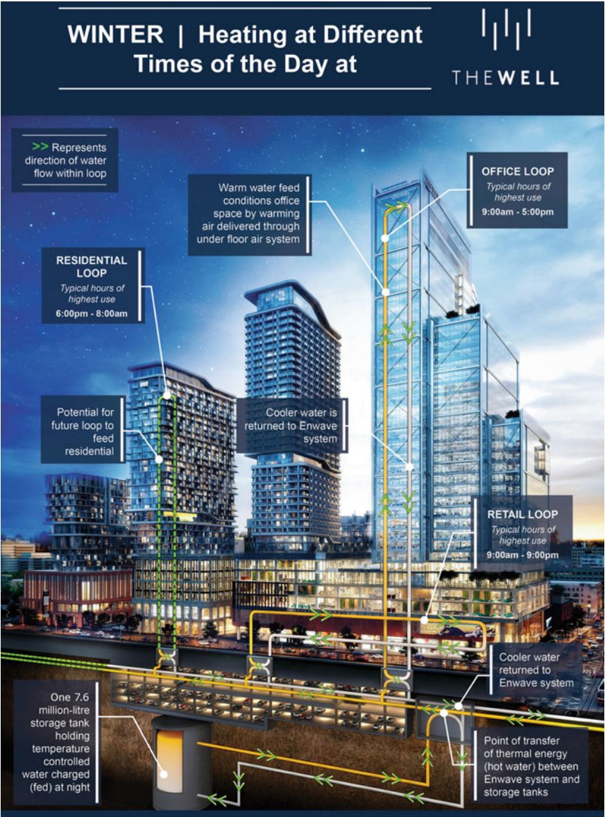
Fig. 1 Winter daytime heating system at the well, per Ref. [1]
