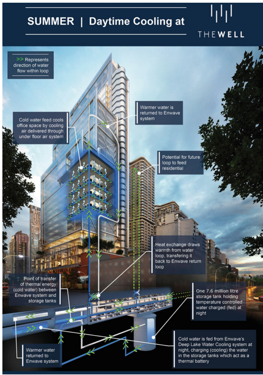
Fig. 2 Summer daytime cooling system at the well, per Ref. [1]
