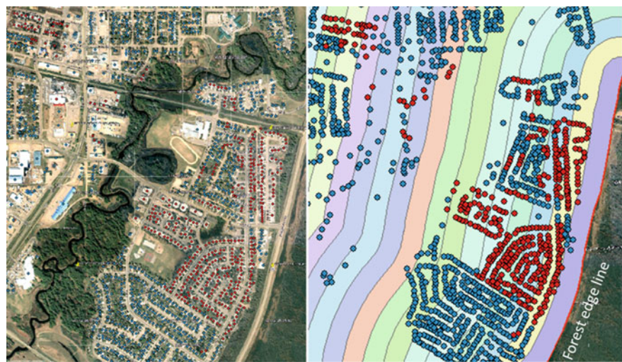
Fig. 5 Extent of damage buildings into the community (left) and forest edge line and considered 100 m wide polygons showing relative distance increments of buildings (right)
