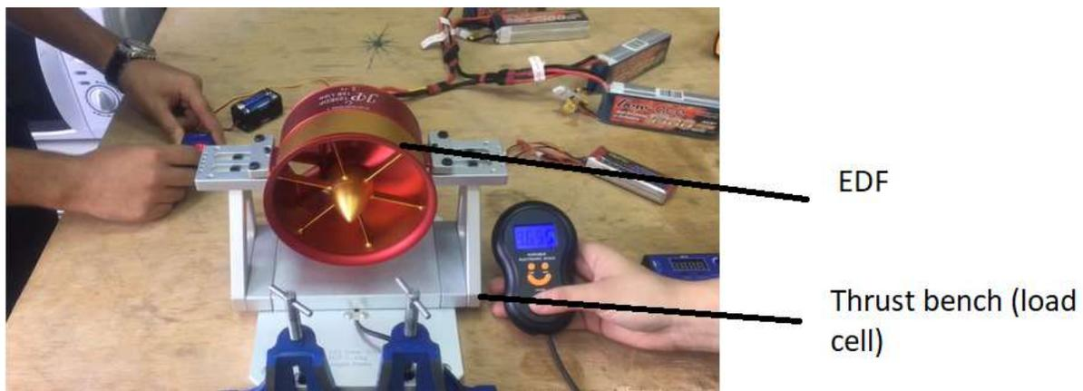
Figure 1. The experimental bench setup
