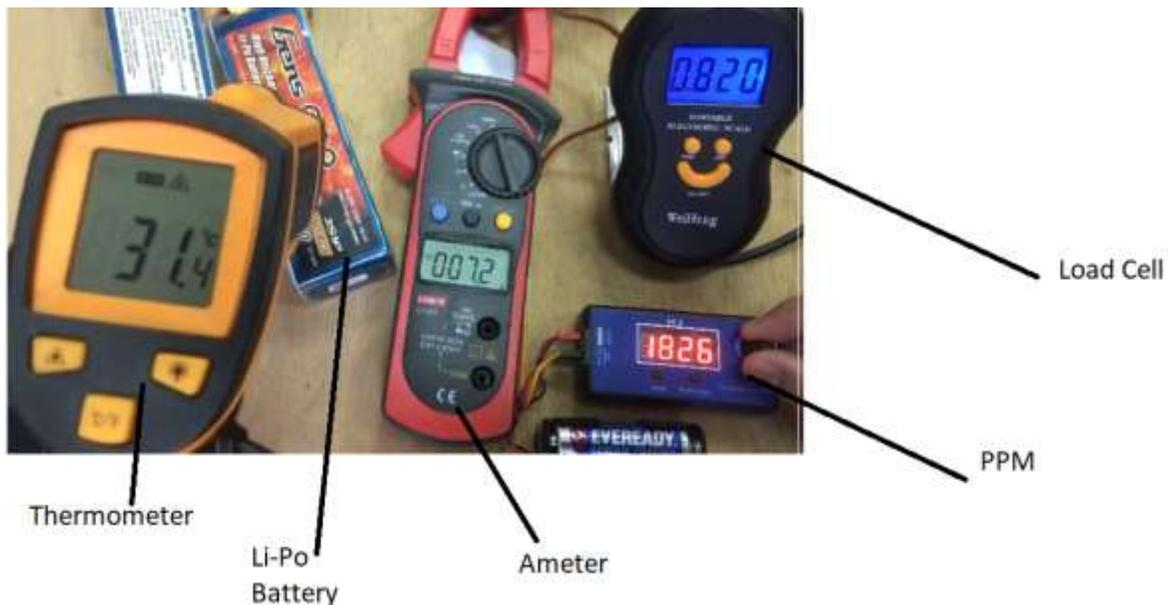
Figure 2. Instruments and transducers that are used to obtain the current, thrust and PPM
