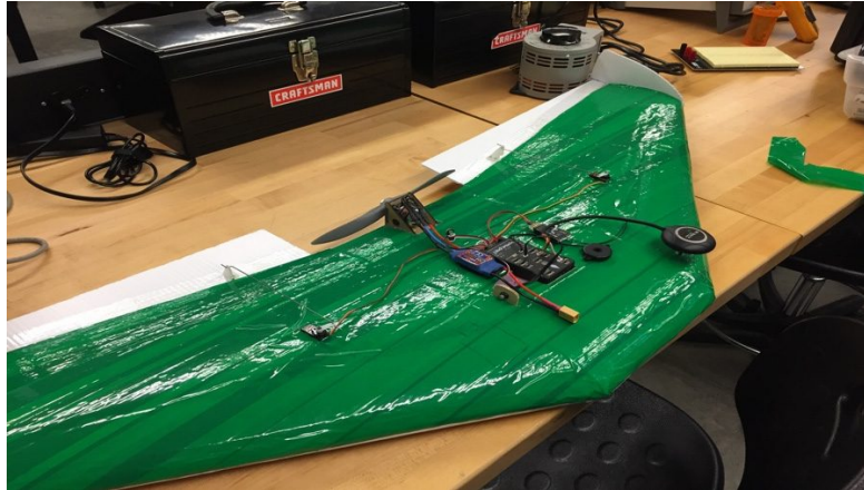
Figure 20. Student foam core design nearing completion with autopilot installed.
