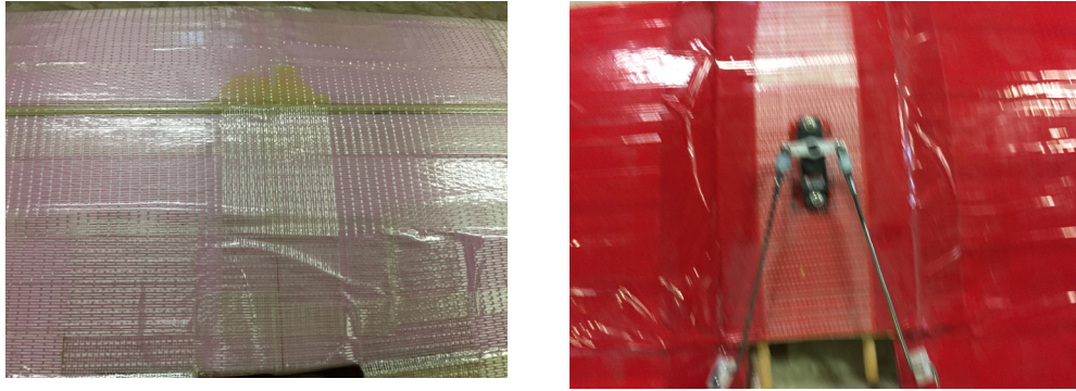
Figure 4. Basic foam wing core with tape reinforcement.
