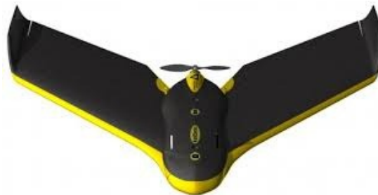
Figure 1. eBee Drone System provided by Parrot. This system is relatively easy to program and fly, and is able to take-off and land with minimal intervention.
