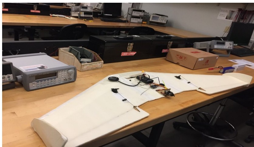
Figure 19. Flight Test design Versa Blunt Nose with student installed Pixhawk autopilot.
