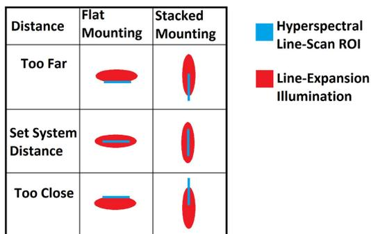
Figure 7. Alignment of imaging and illumination fields as a function of distance from the optics and the positioning of the laser relative to the camera.
