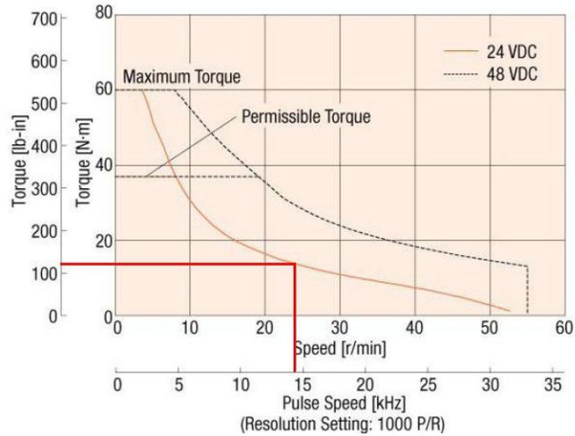
Figure 4. Torque-Speed chart for stepper motor, red line indicates the maximum torque the stepper motor can produce at 22.33 rev/min when powered by 24 VDC.
