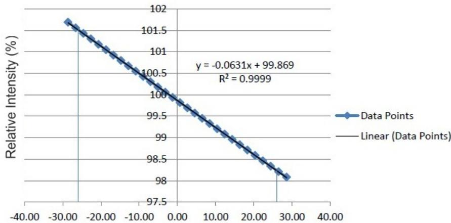
Figure 9. Relative intensity of the illumination profile as a function of distance (inches) from the centerline of the camera. The two blue vertical lines represent the outer edges of area encompassing a 40 inch wide crop row bounded by a 6 inch border on each side of the crop row.
