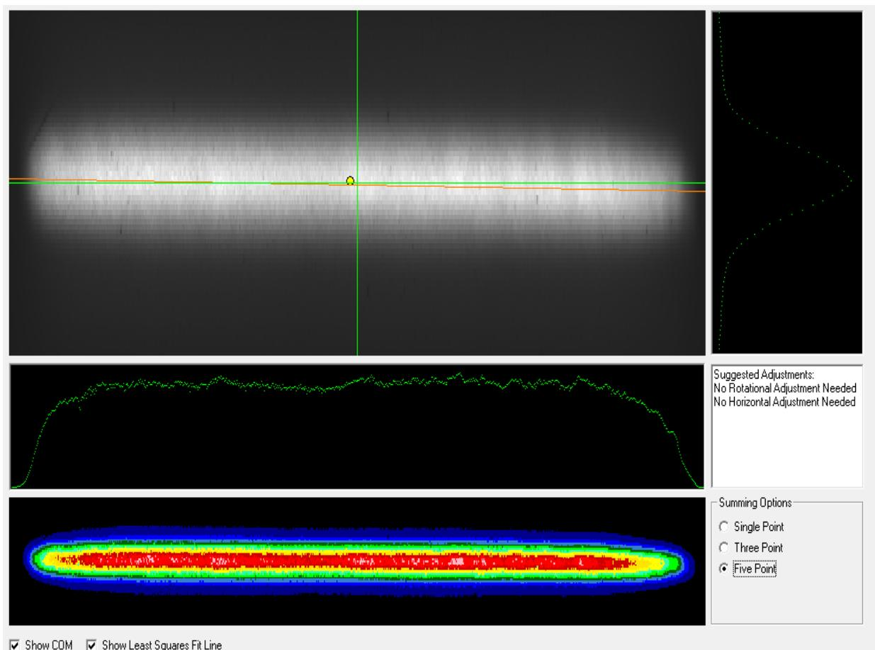
Figure 3. The bottom figure shows a false color image of the illumination profile for single laser pulse using the Powell lens. The five point average across the center of the profile that is displayed immediately above the false color image demonstrates the uniformity of the profile.
