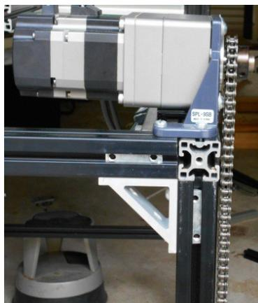
Figure 6. Motor mount and drive.
