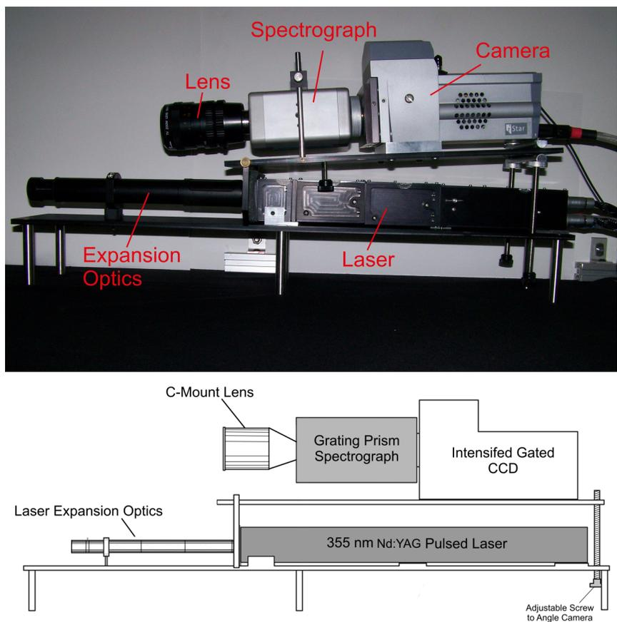
Figure 1. Laboratory based hyperspectral, laser-induced fluorescence, line-scan imaging system.
