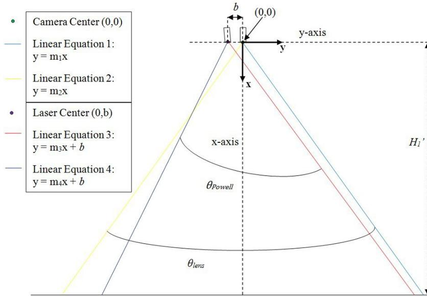
Figure 8. Imaging and illumination fields and equations when the camera lens' center is assumed to be at the origin. The laser lens' center is assumed to be along the y-axis and at an offset  $b$  from the center of the camera lens. Note  $m_1 = \tan(\theta_{lens} / 2)$ ,  $m_2 = \tan(-\theta_{lens} / 2)$ ,  $m_3 = \tan(\theta_{laser} + \theta_{Powell} / 2)$ , and  $m_4 = \tan(\theta_{laser} - \theta_{Powell} / 2)$  with  $\theta_{laser}$  being the angle of the laser relative to the camera.
