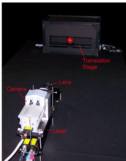
Figure 2. As hyperspectral data is acquired using line-scan images, a translation stage is used to incrementally move objects in front of the system. For field use, the imaging system will be mounted on a cart that moves through produce fields.
