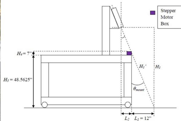
Figure 5. Left, photo of cart. Right, schematic of cart showing dimensions and variables used for imaging field calculations.
