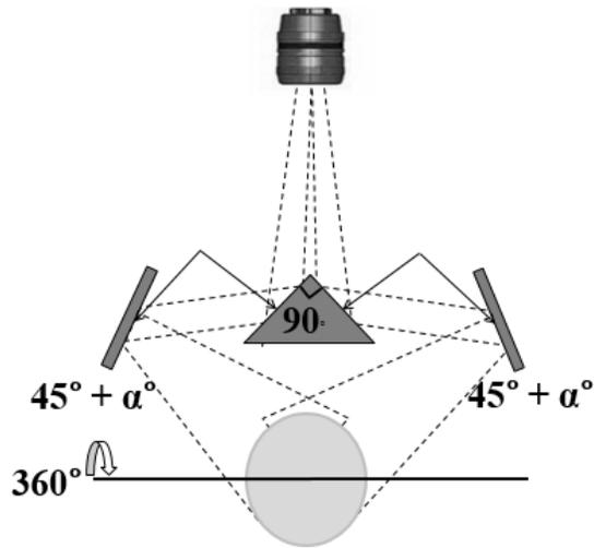
Figure 2. Schematic of the method for simultaneously capturing two side-view line-scan images of a round object
