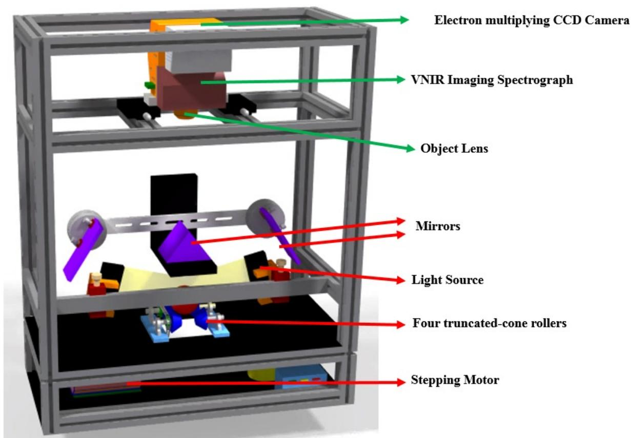
Figure 1. Schematic of hyperspectral imaging-based round-object imaging platform.
