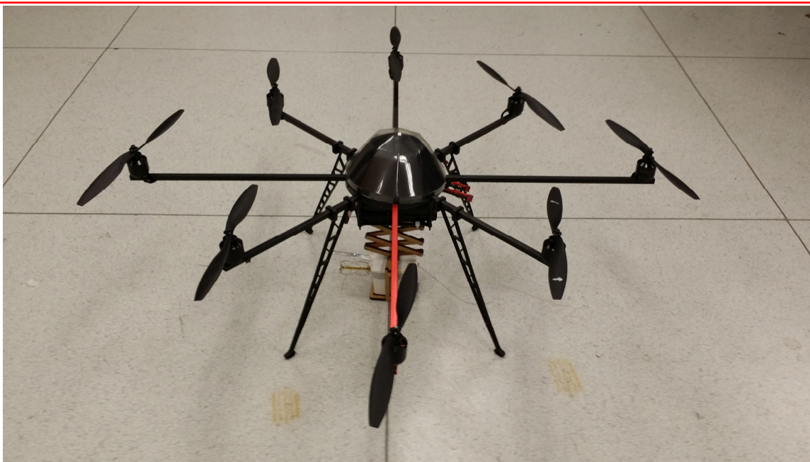
Figure 2. The proposed UAS setup for collecting atmospheric samples and data.
