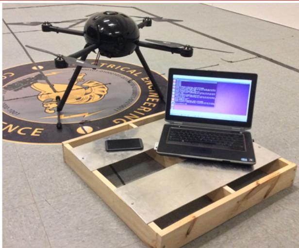
Figure 1: VTOL-ISR prototype vehicle during flight tests inside an indoor GPS-simulated environment. Picture shows quadcopter, charging station, base station (laptop), and user interface (phone or tablet).
