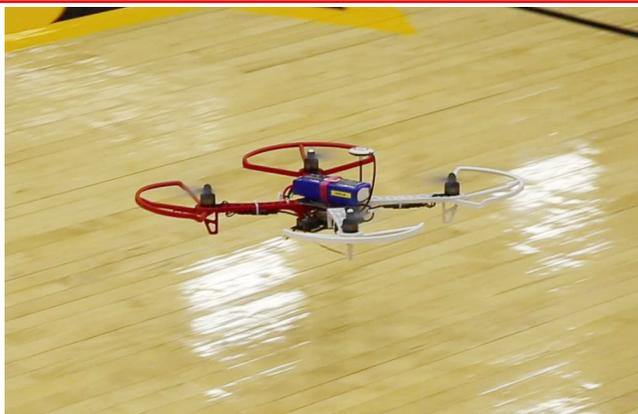
Figure 1. A quadrotor made by DJI (F450) with propeller guards.
