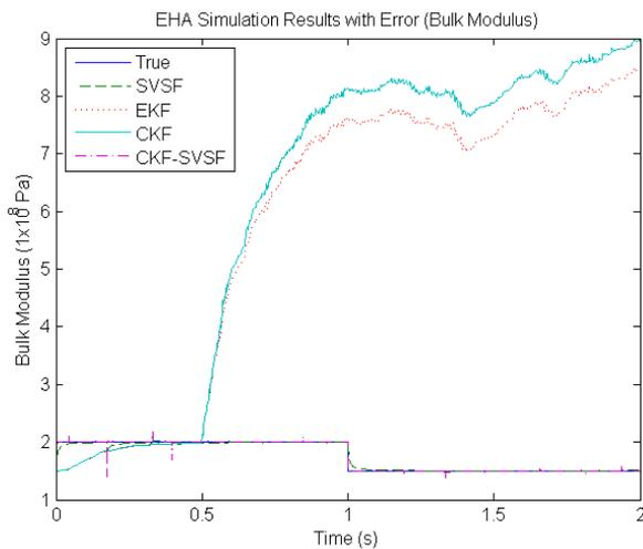
Fig. 5. The bulk modulus estimates for the EHA simulation with modeling error are shown in the above figure.
