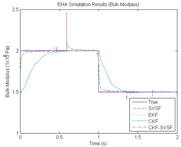
Fig. 3. The bulk modulus estimates for the EHA simulation are shown in the above figure. Note that the EKF and CKF estimates are nearly the same and thus are relatively difficult to distinguish.
