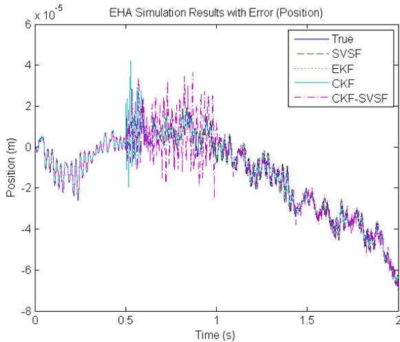
Fig. 4. The position estimates for the EHA simulation with modeling error are shown in the above figure.
