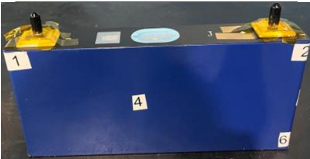
Figure 20 CALB L221N113A Cell with M6 stud terminals.
