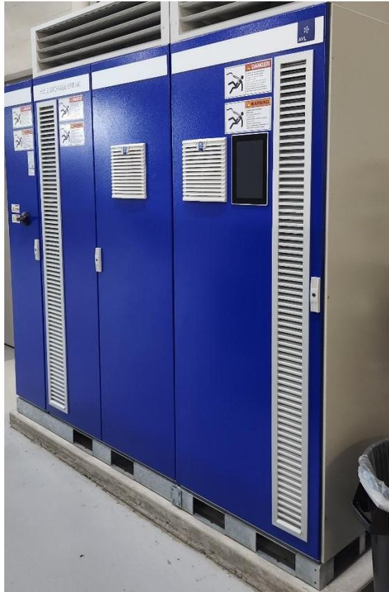
*Figure 69 AVL E-Storage BTE 160 Battery tester and emulator.*
