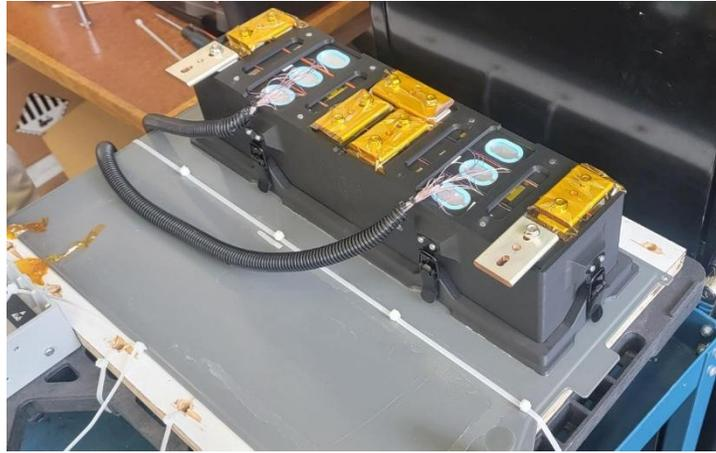
Figure 49 Bottom Cooling Setup final assembly with the top removed.
