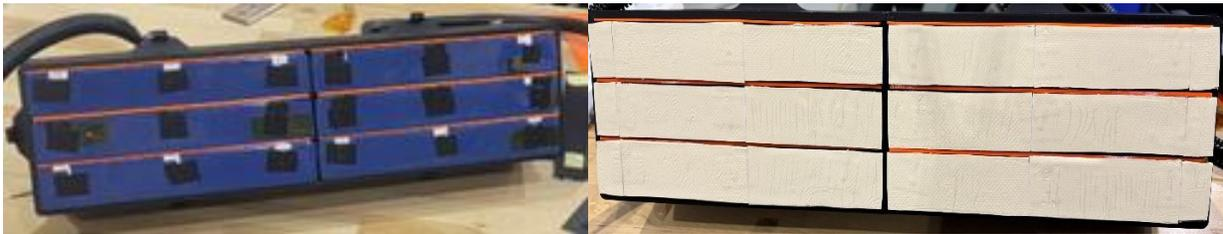
*Figure 47 Bottom Cooling setup TIM installation.*
