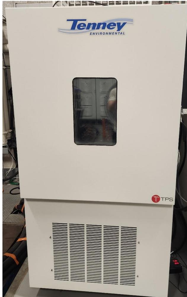
*Figure 70 Tenny Environmental TC20 thermal chamber.*
