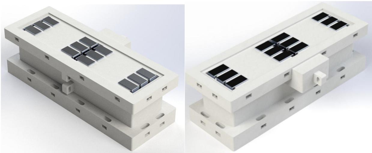
*Figure 115 New testing setup with the MCHP Top attachment to be bonded to the cold plate.*
