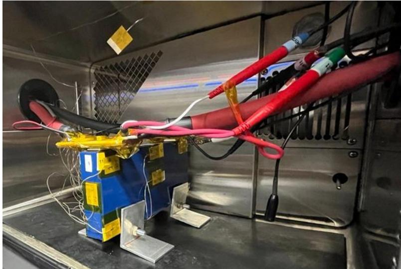
*Figure 23 Single-cell fixture inside the BTZ-133 thermal chamber.*
