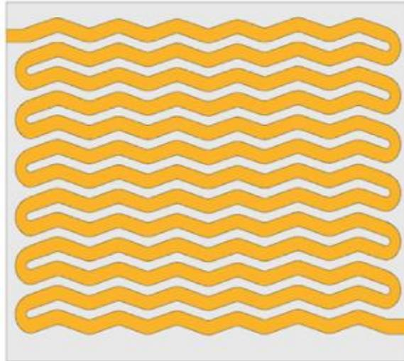
*Figure 17 Zig-Zag serpentine 13-channel cold plate design [97].*
