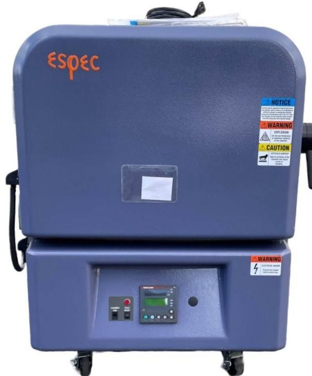
*Figure 21 ESPEC BTZ-133 thermal chamber.*
