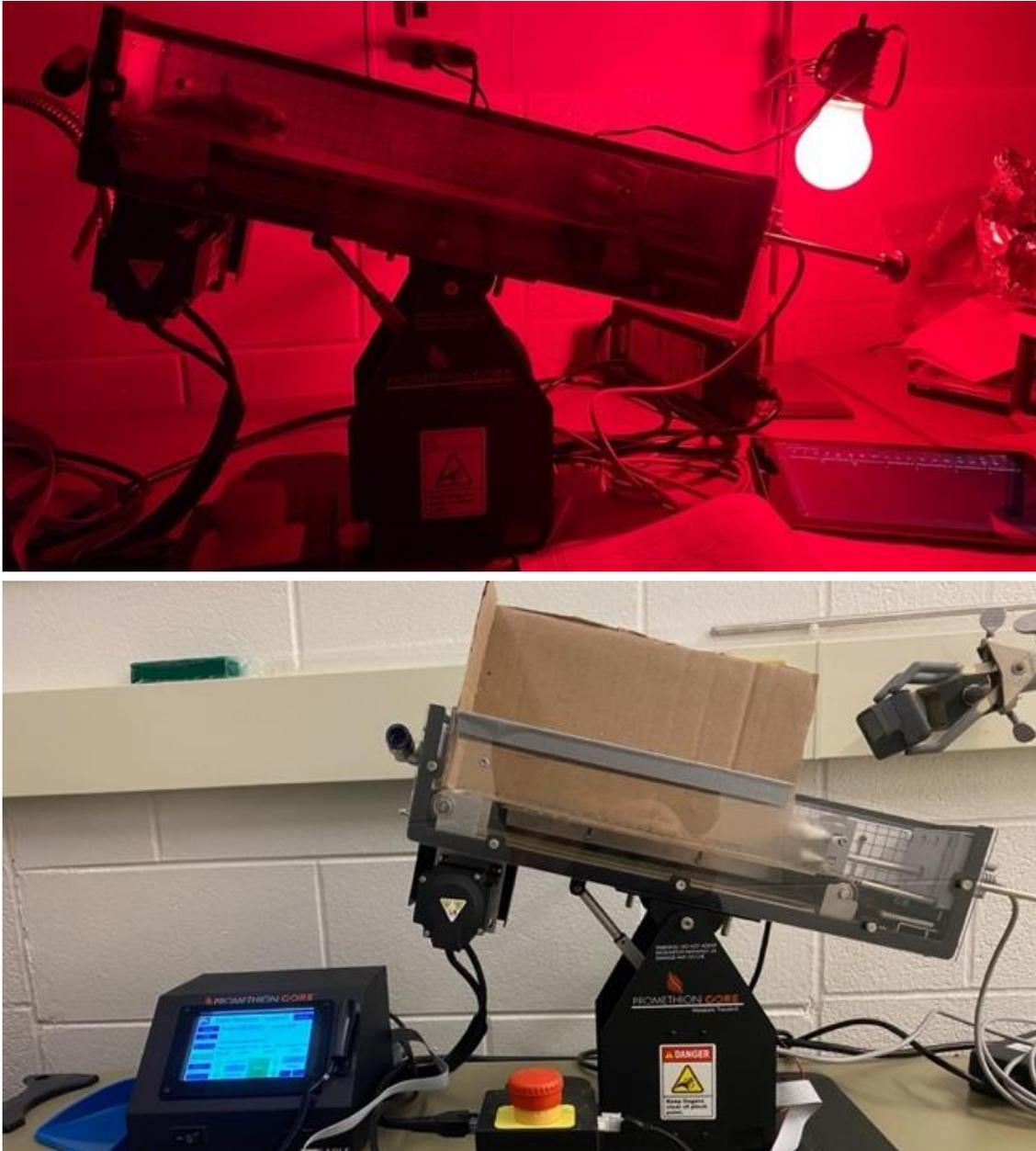
**Fig. 2.** Treadmill used to encourage bats to perform crawling exercise set at 15-degree incline. **(A)** Lateral view of setup for *Pilot Studies* with red light positioned near the treadmill's back end. **(B)** Lateral view of setup for *Experiment 2* with overhead white lighting. A Hero5 GoPro camera positioned above the treadmill was used to record trials.
