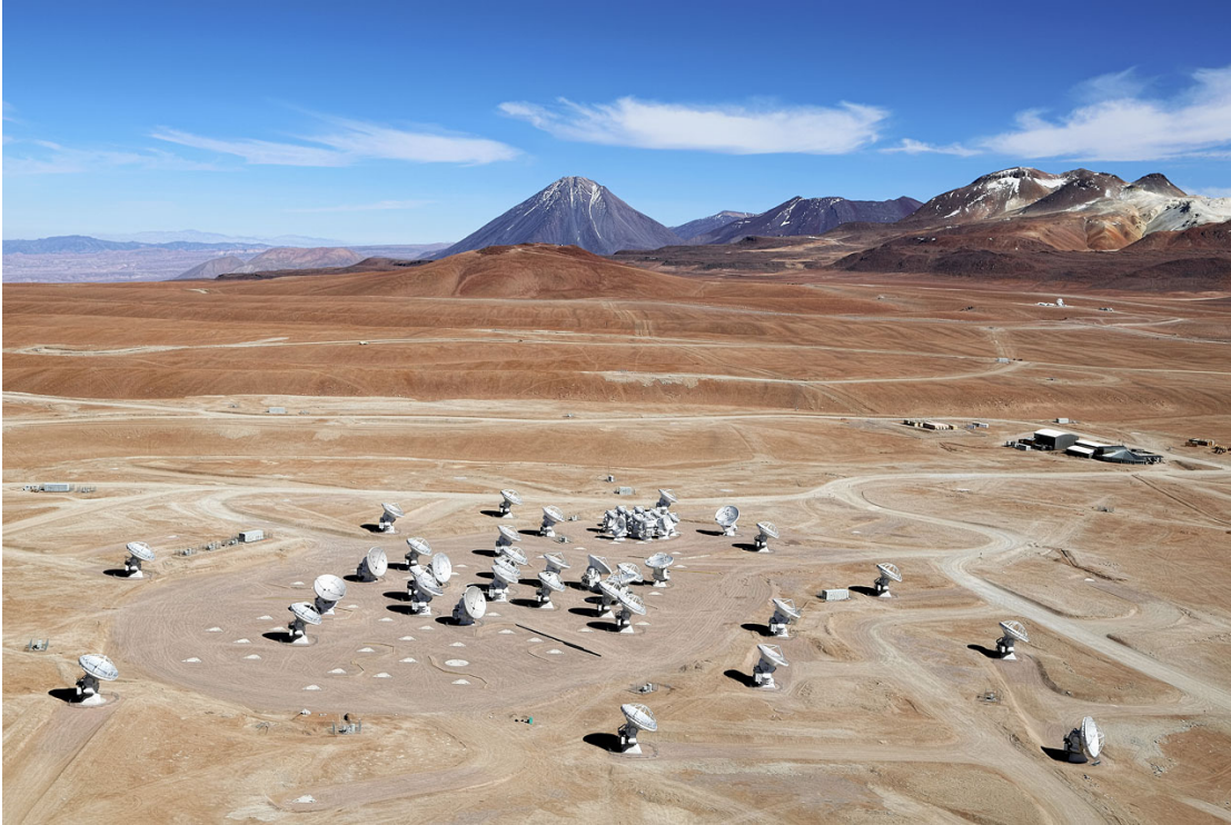
FIGURE 1.8: The ALMA telescope array situated on the Chajnantor plateau in the Atacama desert in northern Chile. The ALMA site is perfect for submillimeter observations as it is far from light and radio pollution, in a dry desert climate, and at an altitude of 5000 m, significantly reducing the precipital water vapour in the atmosphere. Image credit: Clem & Adri Bacri-Normier (wingsforscience.com)/European Southern Observatory (ESO).
