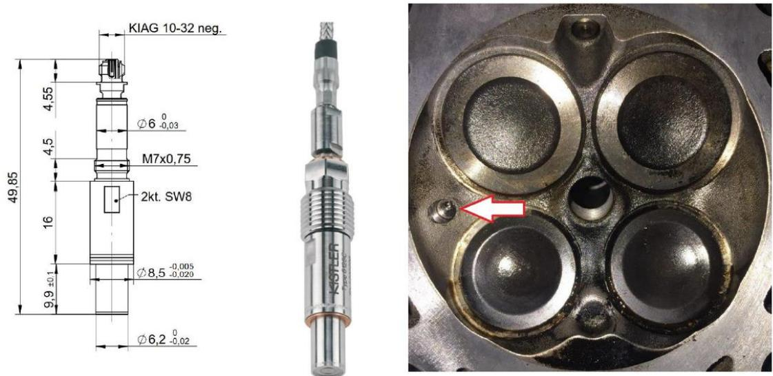
Figure 3.6 Kistler 6125C pressure transducer (left) and combustion chamber location (right)
