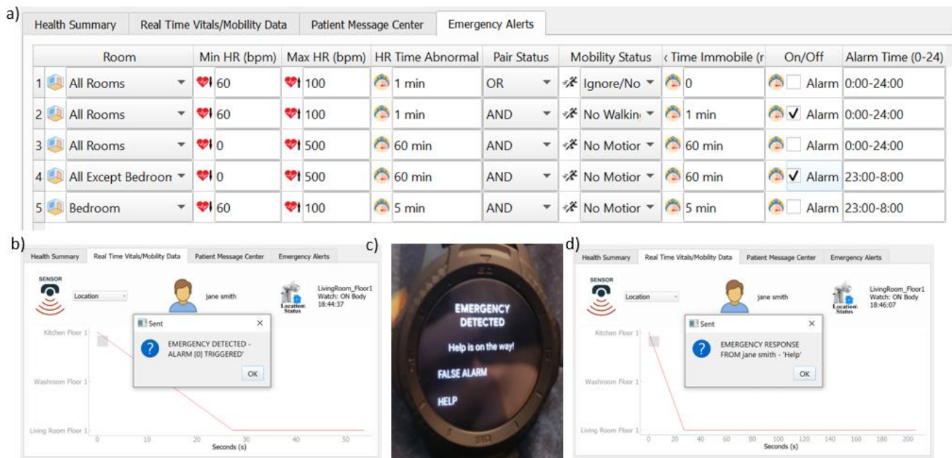
Figure 4.5 a) Emergency alert settings for the alarms based on mobility status. b) Alarm being triggered based on location, immobility, time of day, and heart rate requirements being met. c) Patient’s watch being prompted for feedback to inform them of the alright and confirm if it is an emergency. d) Response from patient being relayed to the healthcare provider via the desktop application. Note that the check-boxed alarms are the context-unaware ones used on one of the watches and the unchecked alarms are the context-aware alarms set on the other watch.
