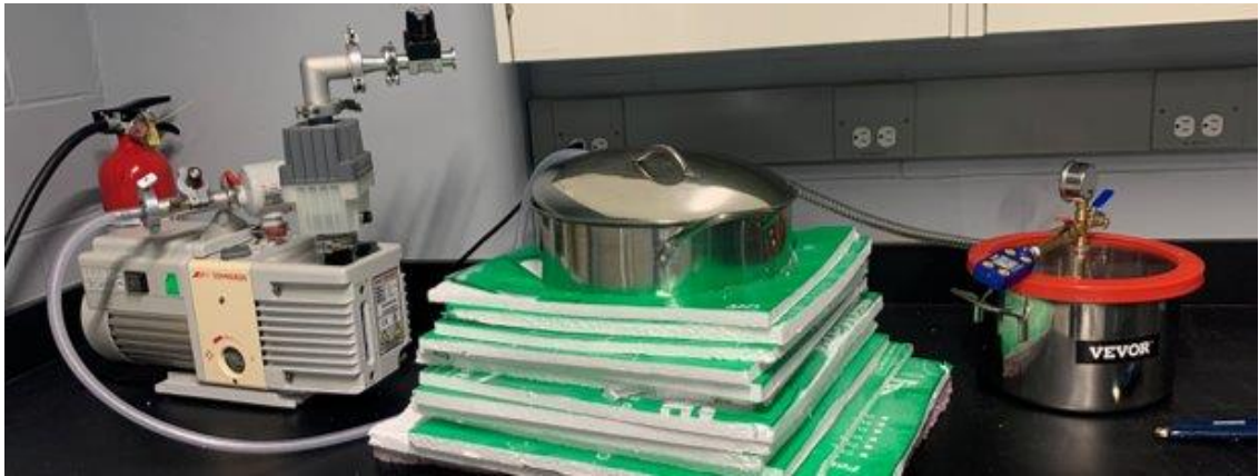
Figure 34. Setup of constructed freeze-dryer. Left to right, Edwards vacuum pump, condensing chamber, sample chamber.
