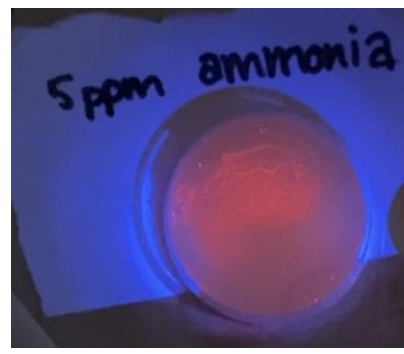
Figure 17. Fluorescence quenching caused by 5ppm ammonia under 385nm light.
