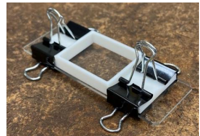
Figure 22. Microscope slide with binder clips, mold for hydrogel casting.
