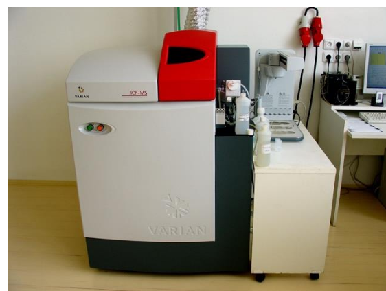
Figure 2.23: Image of the ICP-MS machine used in laboratories to determine sample compositions.
