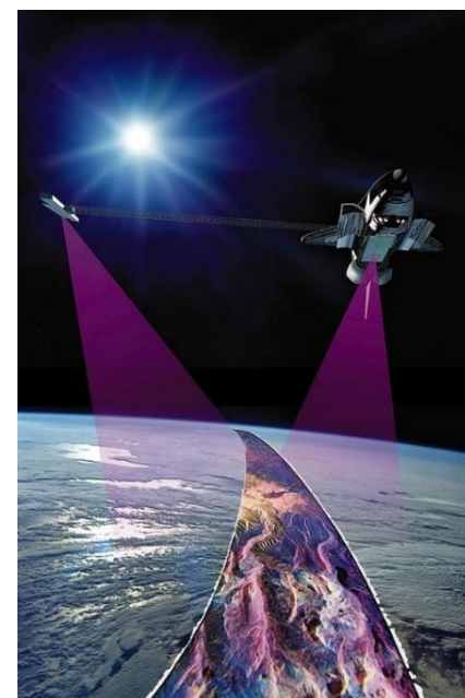
Figure 3.26: Illustration of the Shuttle Radar Topography Mission. Launched in 2000, this shuttle used two radar antennas to sweep the surface of the Earth in 10 days to obtain extensive, high-resolution data of the Earth's topography.
