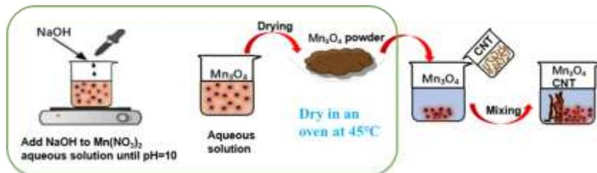
Figure 4- 1 Chemical synthesis of  $\text{Mn}_3\text{O}_4$ .
