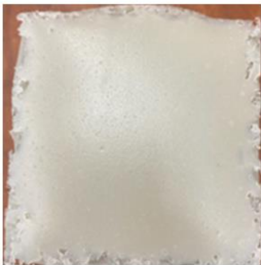
Figure 8.2. Photo of a rotomolded box processed using: (A) 100% powder obtained via the grinding mill with a 0.5 mm sieve of extruded sample “ANT” and (B) a blend of 70 wt% virgin RG8660 powder and 30 wt% of ground “ANT” powder obtained from the grinding mill
