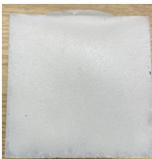
Figure 8.2. Photo of a rotomolded box processed using: (A) 100% powder obtained via the grinding mill with a 0.5 mm sieve of extruded sample “ANT” and (B) a blend of 70 wt% virgin RG8660 powder and 30 wt% of ground “ANT” powder obtained from the grinding mill
