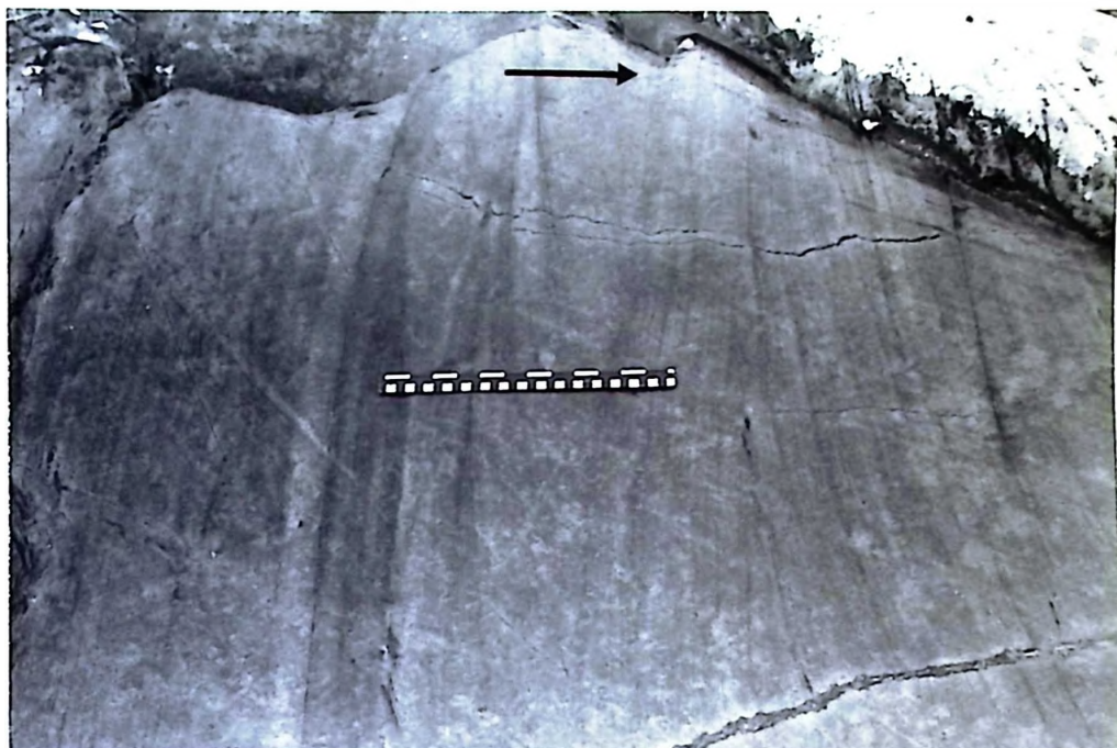
Figure 28. Low angle trough cross-bedding within fine to medium grained arkosic sandstone. Arrow indicates top direction to the north. Scale in inches and centimetres. Island B, Vermilion Lake.
