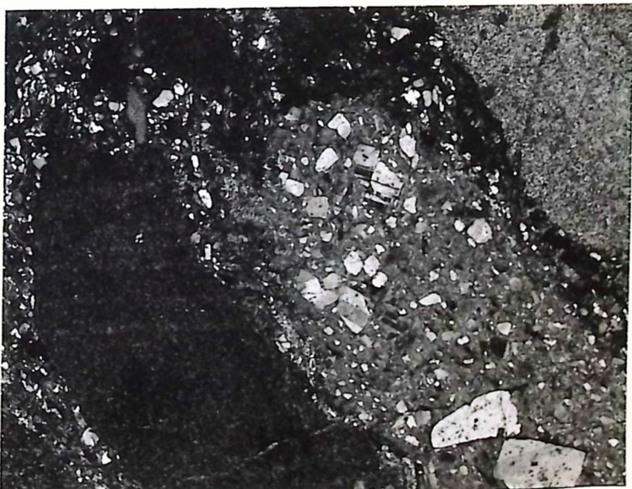
Figure 73. Projection print of a thin section of granite-bearing conglomerate with arkose matrix surrounding dark basic rock fragment, felsic tuff fragment, and acidic volcanic fragment (upper right). Note the cracked plagioclase grains in the tuff. Field of view is 1.4 cm wide.
