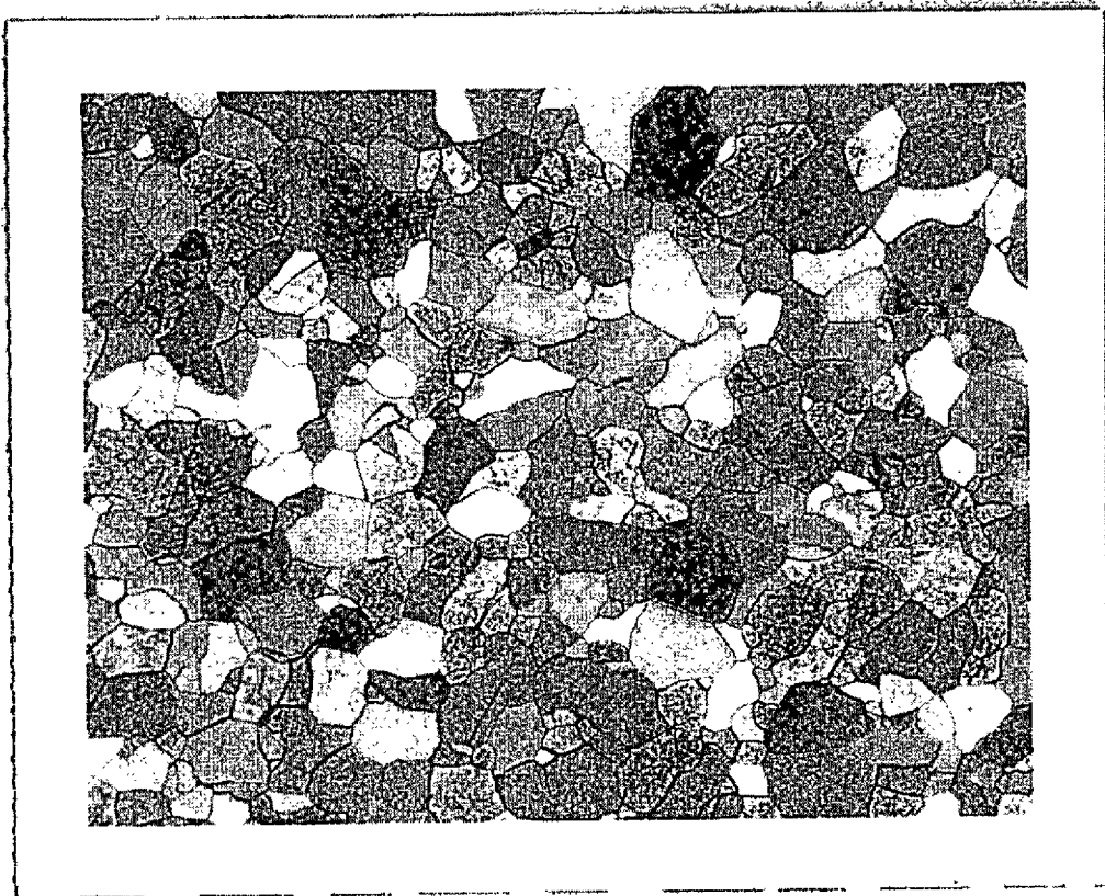
Figure 4.18 The Stage Zero Sample with the Equi-cored Grains in the Longitudinal Plane
