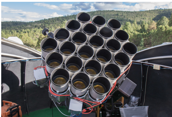
Figure 3.1: The Dragonfly Telephoto Array. This image shows 24 of the 48 telephoto lenses and CCD cameras.
