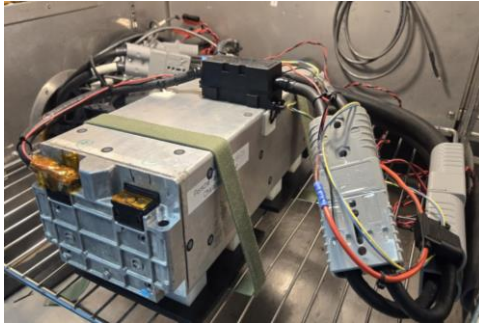
Figure 3.5: Cell characterisation test setup inside chamber
