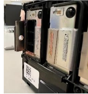
Figure 3.6: Cell 1 tab separated from the rest of the module
