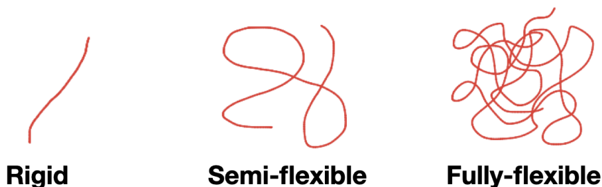
FIGURE 1.2: Illustration of polymer chains with varying degrees of flexibility.
