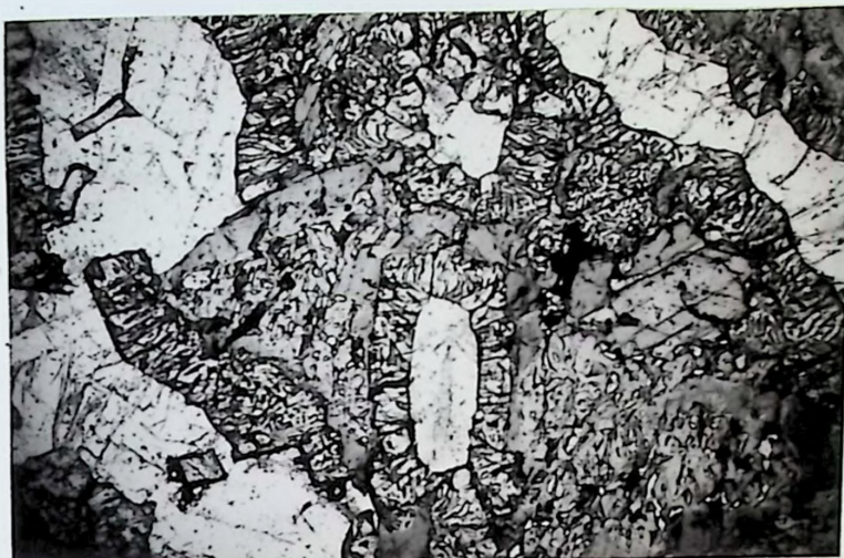
Plate 5-14 Corona of myrmekitic epidote on amphibole - plane. In this case the primary pyroxene has been completely uralitised to an amphibole/quartz symplectite. Note regularity with which epidote rims this secondary uralite.
