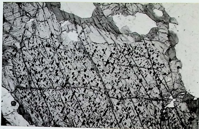
Plate 5-4 Oxide exsolution in clinopyroxene - plane. Note here that oxides are restricted to large central unrecrystallised portion. Rimming this is area of small, recrystallised grains free of oxides - light gray area; this is, in turn, rimmed by amphibole - dark grey. Although section is such that pyroxene cleavage is not at 90^\circ , note that orientation of oxides is at 45^\circ to cleavage.
