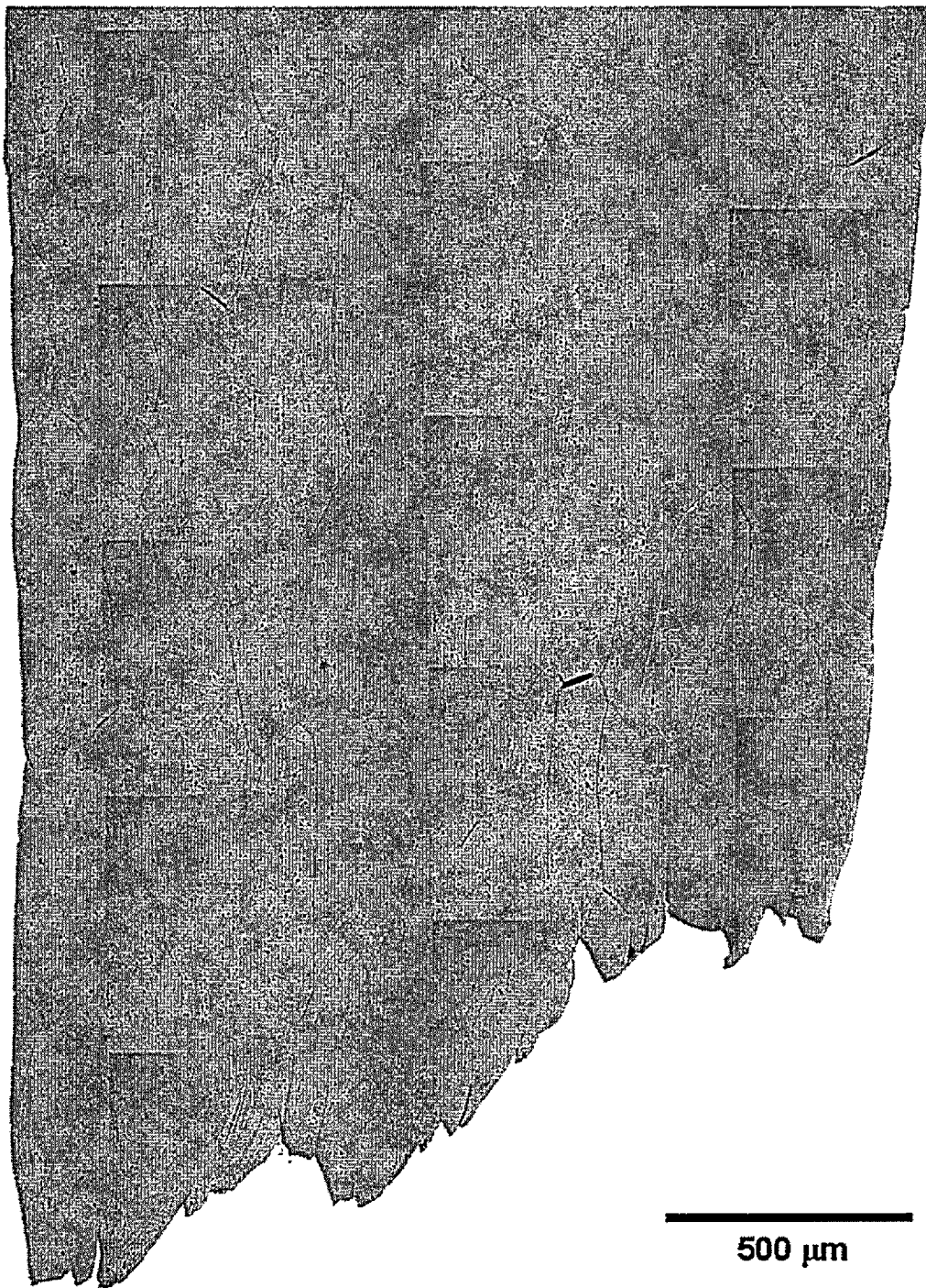
Figure 4.87: Low-Fe 6111 T6 sample tested at 125 MPa etched and viewed to reveal shearing and slip.
