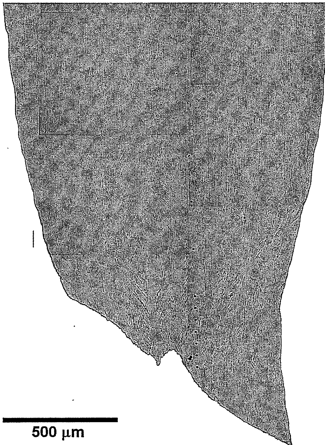
Figure 4.24: Low-Fe 5754 sample tested at 0.1 MPa and 77 K, etched to reveal shearing and slip.
