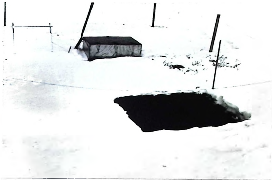
Plate 11. Winter view of experimental site. Note straw mulch, and snow cleared plots, and thermocouple ladder.
