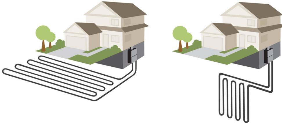
(a) Horizontal ground heat exchanger      (b) Vertical ground heat exchanger
