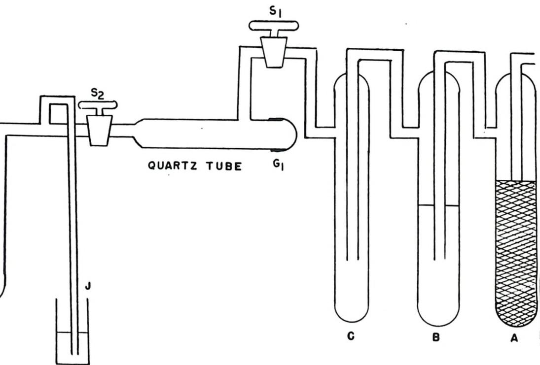
FIG. 3 COMBUSTION LINE
