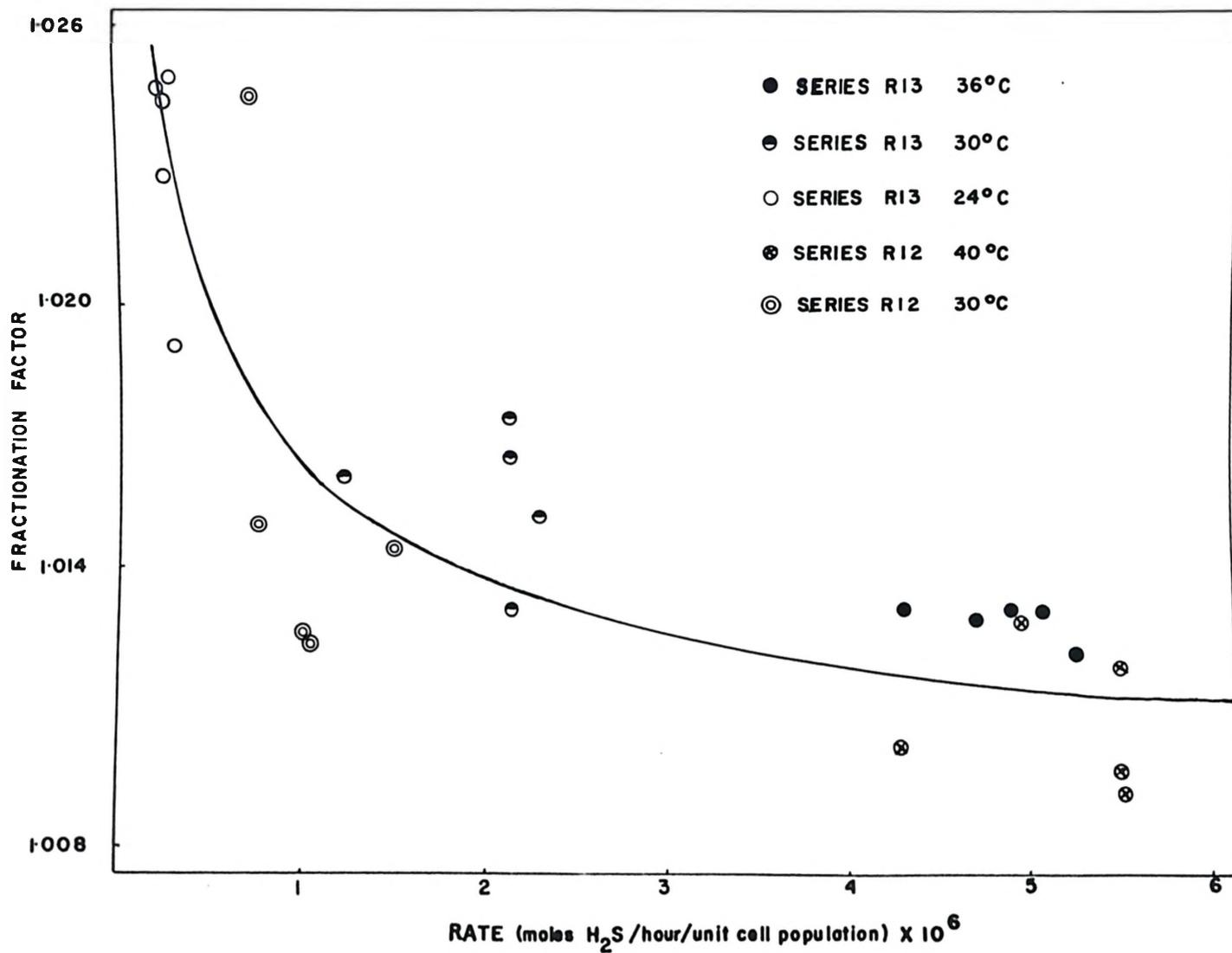
FIG. 6 EFFECT OF TEMPERATURE ON ISOTOPE FRACTIONATION
