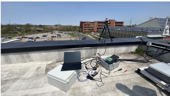
(a) The data collection setup on the MARC rooftop, 12 meters above the road surface.
