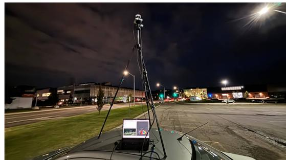
(b) The roadside data collection setup, 3 meters above the road surface.
