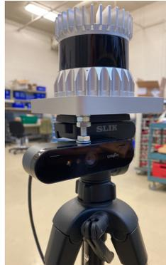
(a) The *Ouster OS1-64* used for data collection with a synchronized camera mounted on a tripod.
