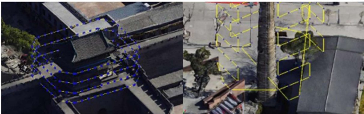
Figure 2.20 UAV path planning to survey the Ancient City of Ping Yao [46]
