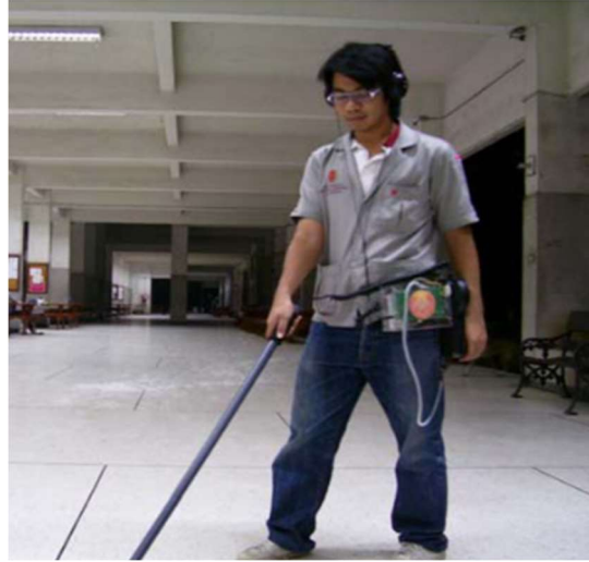
Figure 2.46 The navigation device attached to a user with a headphone and the RFID antenna built-in cane [65]
