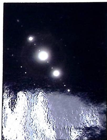
Fig. 11(c) Electron diffraction patterns showing weak super lattice spots (in addition to strong b.c.c.  $a_0 = 3.01 \text{ \AA}$  spots) which can be indexed on the basis of a  $9.05 \text{ \AA}$  simple cube (taken from H-500-3).
