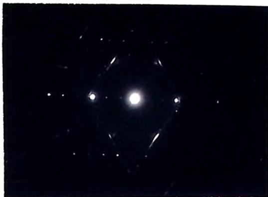
Fig. 11(b) Electron diffraction pattern showing diffraction streaks due to the coherent precipitation of a second phase (taken from H-500-2).
