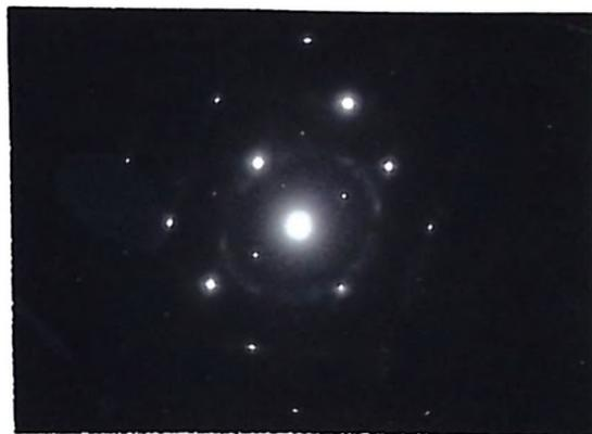
Fig. 10(d) Electron diffraction pattern (typical of the H-700 series) taken at some deviation from the Bragg condition showing diffuse diffraction maxima in addition to the body-centered-cubic CsCl pattern.
