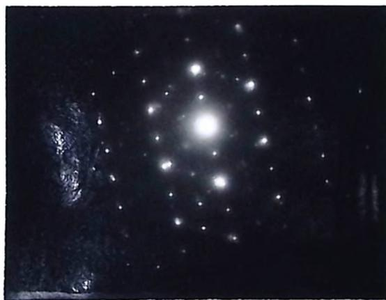
Fig. 17(b) Electron diffraction pattern of the transition phase.
