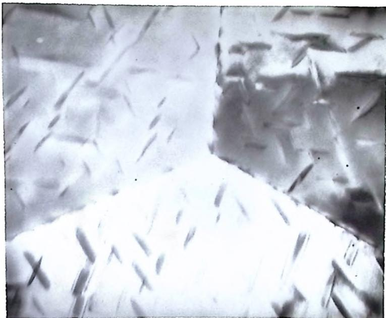
Fig. 11(a) 51% Ni alloy annealed at 700°C for 5385 minutes followed by 460 minutes at 500°C (sample R-500-2) showing coherent precipitates which are presumed to be  $Ti_2Ni$  X 30000
