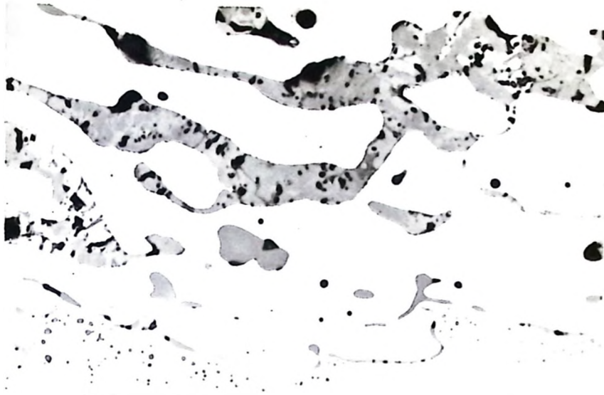
Fig. 36 Photomicrograph of the large areas of iron between the \alpha\text{FeS} - \beta\text{MnS} phases equilibrated at 1300^{\circ}\text{C} for 80 minutes. Note the fine precipitates at the front of the sulphide-iron interface. 800x, Polarized Light
