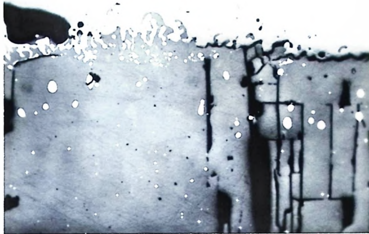
Fig. 24 Typical \beta MnS film on the surface of a levitated specimen. Note the iron precipitates and the non-planar sulphide-iron interface. 800x
