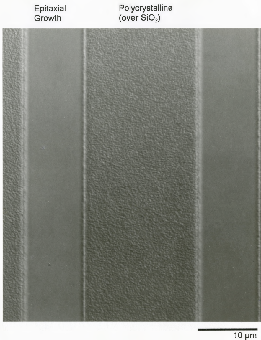
Figure 2.4: Nomarski micrograph of top view of the wafer after growth.
