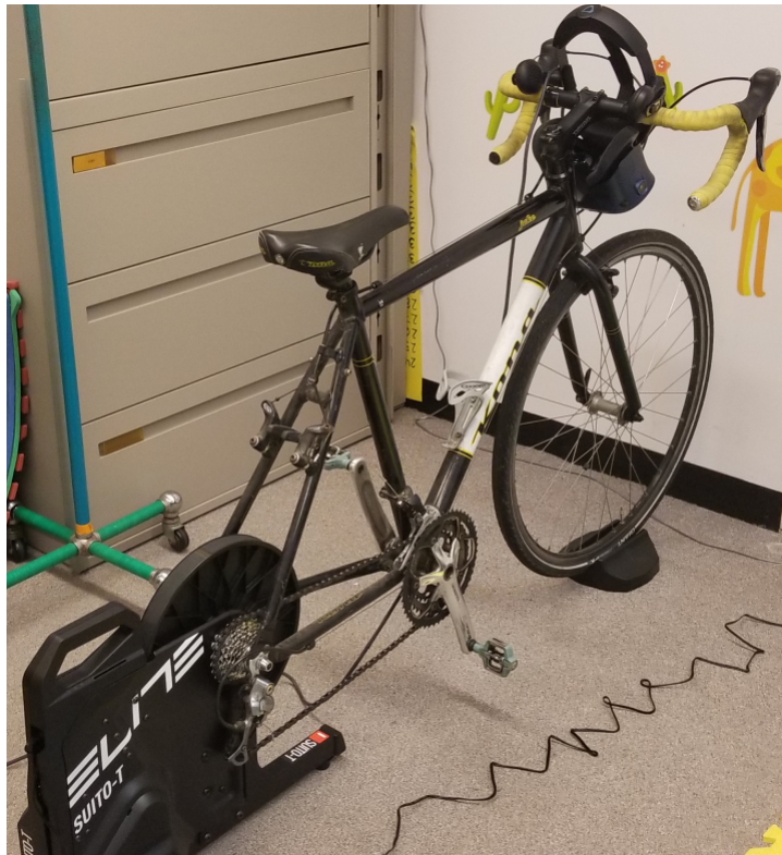
Figure 6.2: Stationary Bike and Trainer setup for Development
