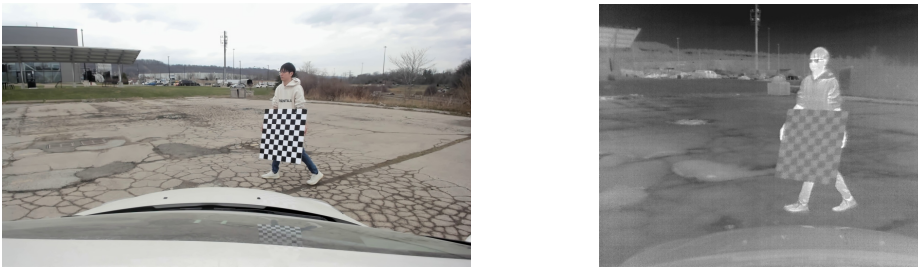
Figure 3.19: Another calibration example with an off-center checkerboard position. It's important to note that LiDAR sensor data is also collected during this time, resulting in the utilization of the same set of image data for computing both intrinsic and extrinsic parameters, as well as distortion.
