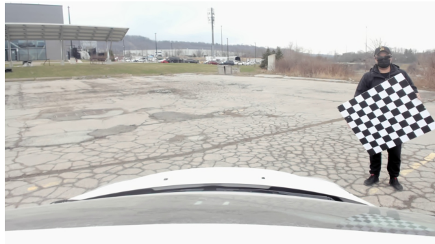
Figure 3.16: Example of a tangential distortion, image is artificially distorted for demonstration purpose.
