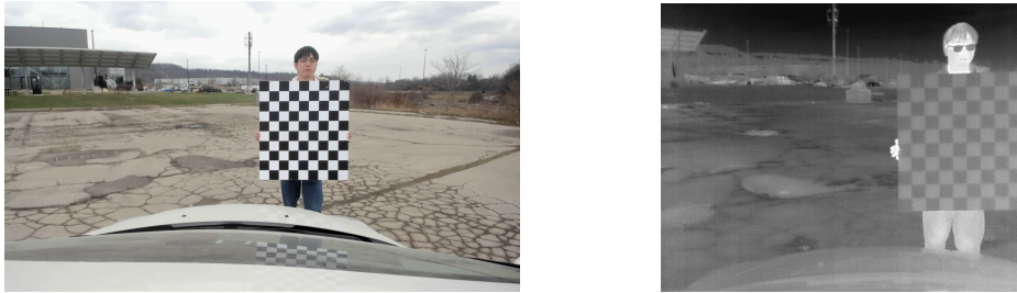
Figure 3.18: A calibration example with the checkerboard close to the centre of the sensor, image to the left is the RGB camera, and image to the right is the IR camera.
