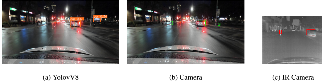
Figure 6.32: Example of YoloV8 missed detection, the pedestrian to the left was not detected. But purposed vehicle perception caught the jaywalking person.
