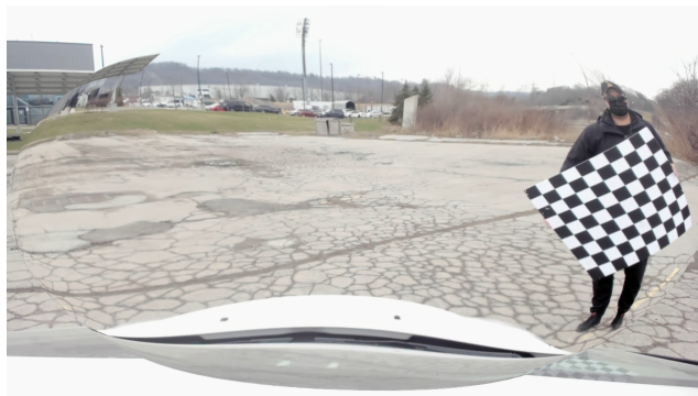
Figure 3.13: Example of a moustache distortion, image is artificially distorted for demonstration purpose.
