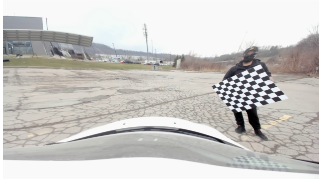
Figure 3.12: Example of a pincushion distortion, image is artificially distorted for demonstration purpose.
