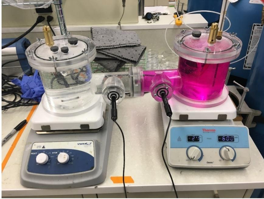
Figure 6. LOC test prior to first use of the device, showing OP tank (no dye) and OR tank (pink dye). The dye test was performed to confirm no passage of micromolecules through the membrane.
