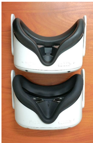
Figure 3. Meta Quest 2 headset with original facial interface (top) and modified silicone light blocking facial interface (bottom).
