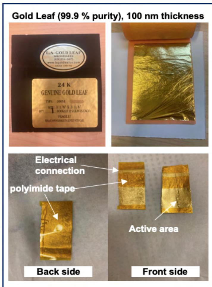
Figure 5.2 Images of the gold-leaf sheets and the fabricated electrode (front and back side).
