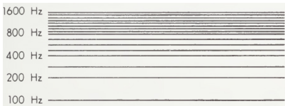
FIGURE 7.1 The Harmonic Structure of a 100-Hz Tone
