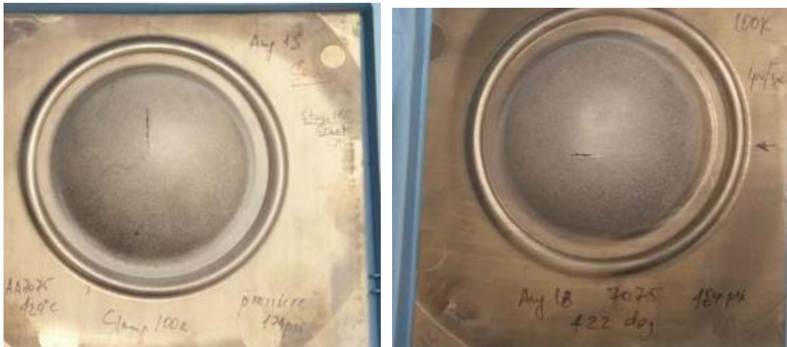
Figure 6-92. Photographs of two bulged samples of baseline 7075 sheet tested at 425°C using Macrodyne press.
