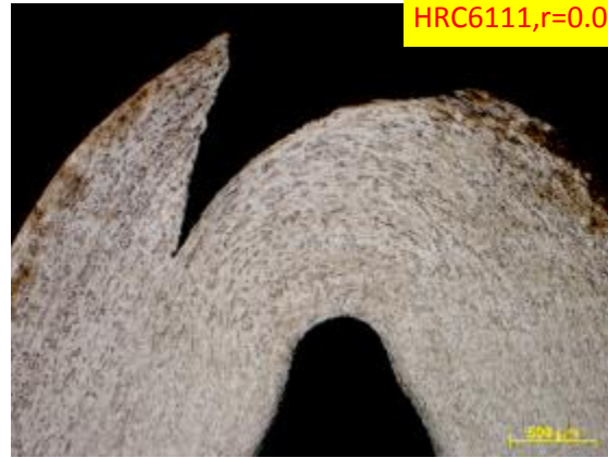
Figure 6-24. A comparison of microstructures of bend specimens of AA6111-T4 and HRC 6111-T4 from tests conducted with different bending mandrel radii.
