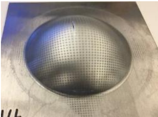
Figure 10-1. Photographs and corresponding Argus major strain maps of various hot air bulge sample of baseline AA6111 sheet.
