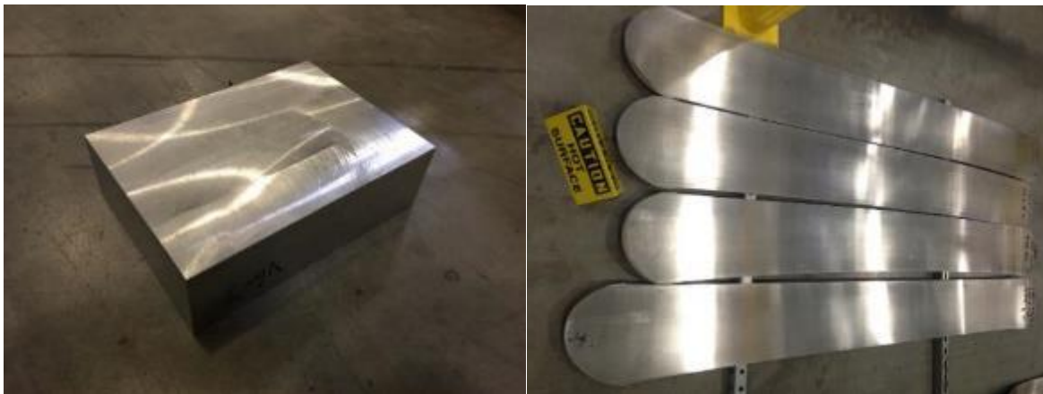
Figure 5-2. Photographs of an ingot sample and the resulting hot band plates from 4 ingots.
