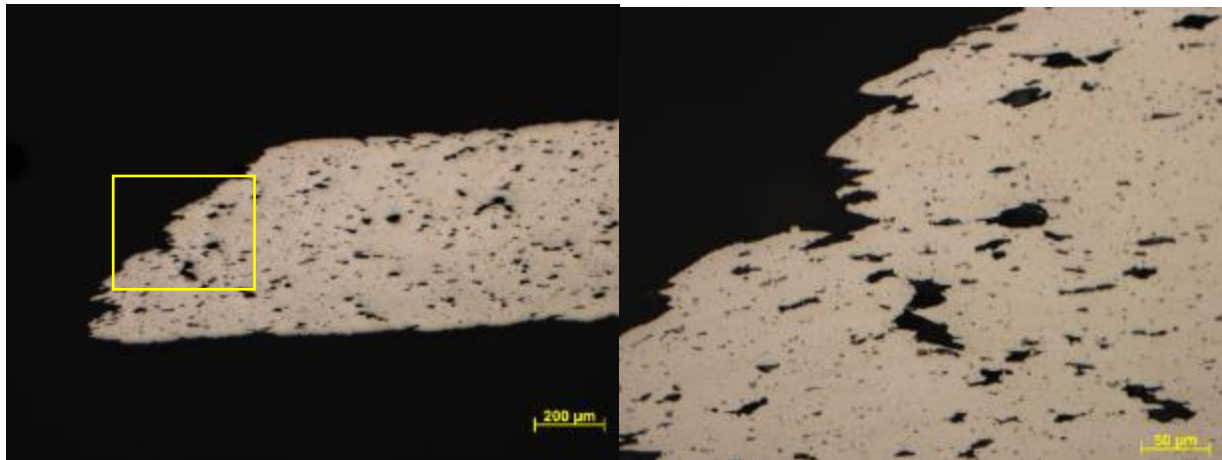
Figure 6-77. Through-thickness optical micrographs at two different magnifications of a AA7075 equi-biaxial hot gas bulge sample tested to fracture at 470°C.
