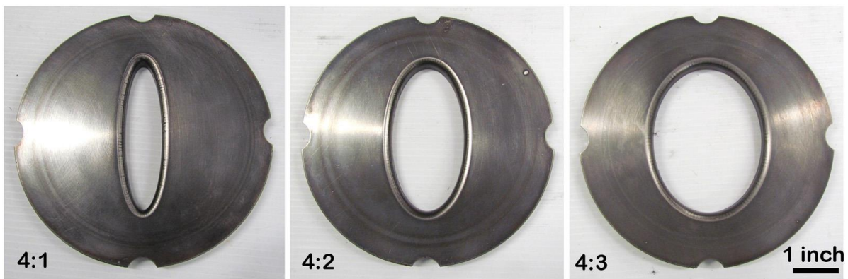
Figure 4-8. Photographs of the dies with elliptical openings for hot gas bulge test.
