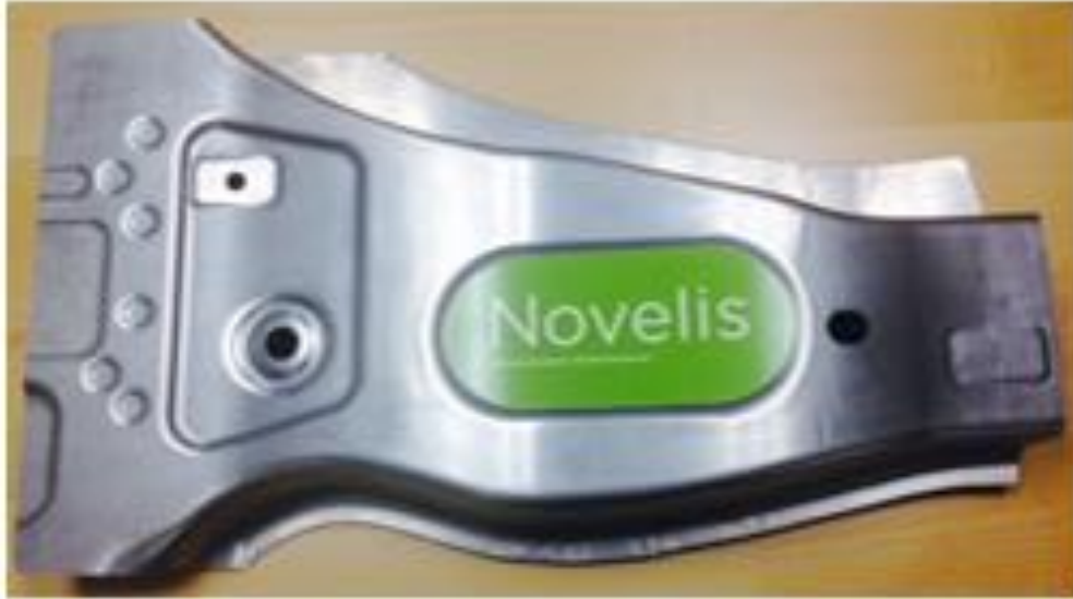
Figure 1-5. A Hot Formed B-pillar reinforcement using Novelis' 7075 aluminum.
