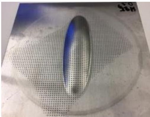
Figure 10-2. Photographs and corresponding Argus major strain maps of various hot as bulge sample of baseline HRC6111 sheet.
