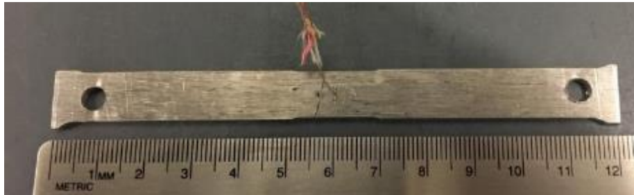
Figure 4-3. A photograph of Gleeble tensile test specimen with a thermocouple welded for elevated temperature test.
