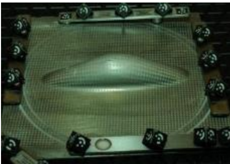
Figure 10-7. Photographs and corresponding Argus strain maps of various hot as bulge sample of MRC 7075 sheet at 425°C.
