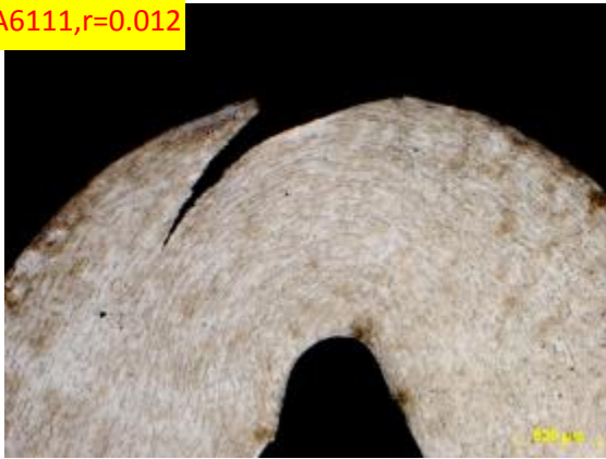
Figure 6-24. A comparison of microstructures of bend specimens of AA6111-T4 and HRC 6111-T4 from tests conducted with different bending mandrel radii.
